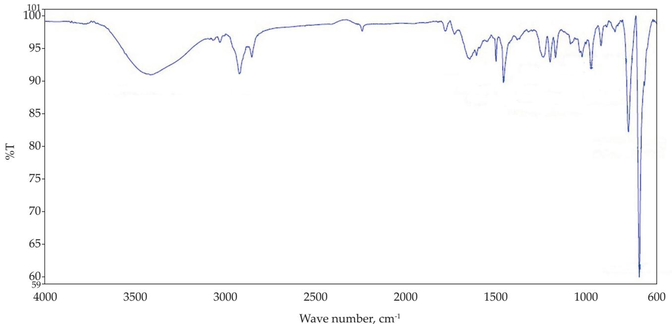
Fig. 3. FTIR spectra of car side mirror cover
