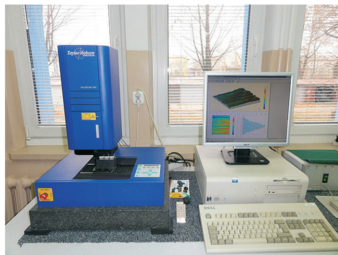
Fig. 1. Views of model printing and measurement process: a) model orientation in the Fortus 360-mc printer space, b) 3D Talyscan 150 profilometer
