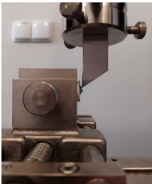
Fig. 2. Testing of bracket-ceramics bonding strength
