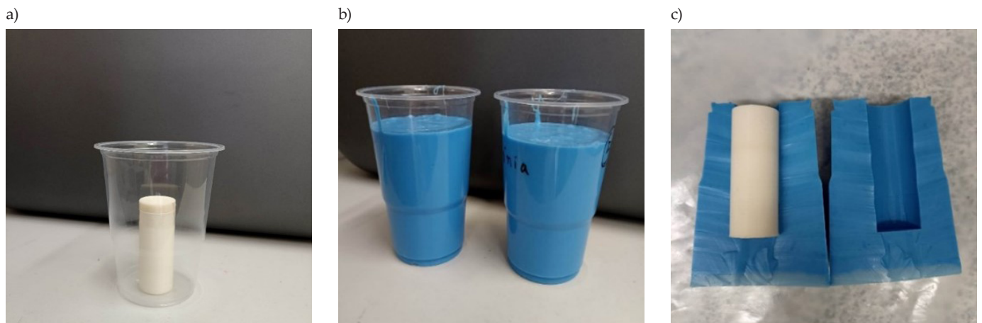
Fig. 3. Stages of obtaining a silicone mold: a) a model printed from ABS attached to the bottom of the cup, b) a cup with 3D model filled with silicone, c) a silicone mold with the model inside
