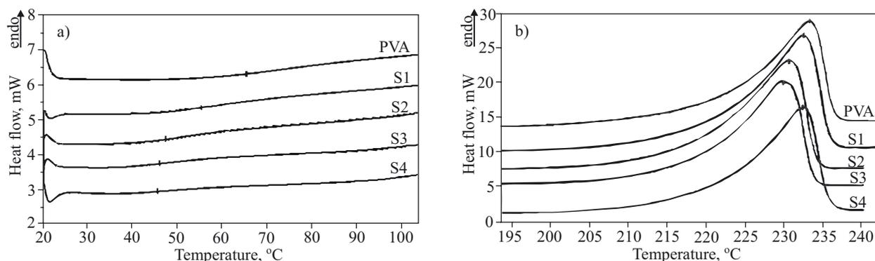
Fig. 5. The DSC thermograms for PVA and PVA/β-CD membranes at temperature ranges: a) 20–100 °C, b) 195–240 °C
