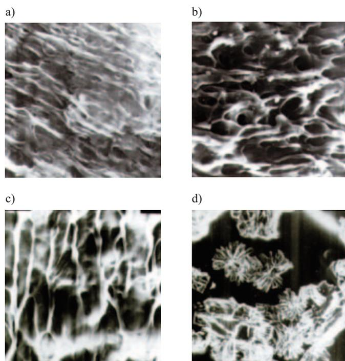
Fig. 1. The SEM images of the PVA and its blends with  $\beta$ -CD: a) PVA, b) sample S1, c) sample S2, d) sample S4
