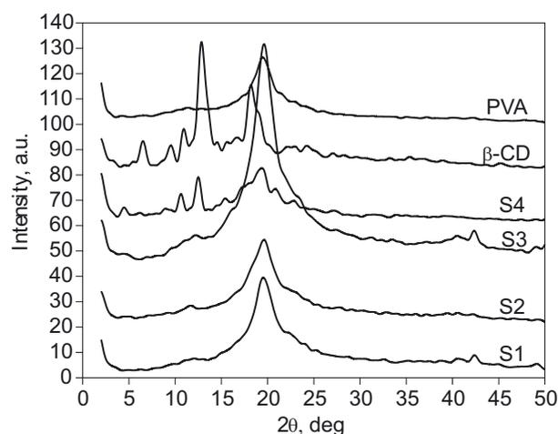
Fig. 2. The XRD diffractograms of the membranes of PVA,  $\beta$ -CD and their blends (samples S1 – S4)
