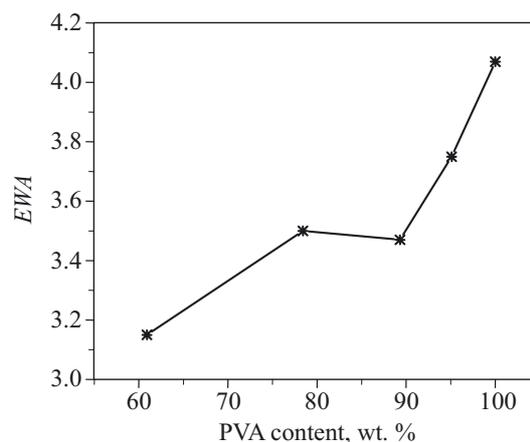
**Fig. 4.** Equilibrium water absorption (EWA) at 37 °C versus PVA content in PVA/ $\beta$ -CD membranes
