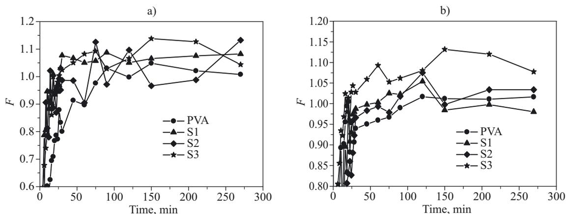
**Fig. 3.** Swelling fraction ( $F$ ) curves as a function of time for PVA and PVA/ $\beta$ -CD membranes at the temperature of: a) 25 °C, b) 37 °C
