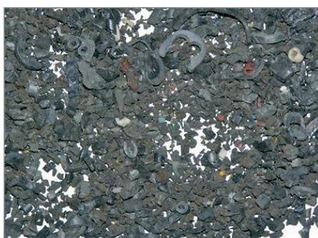
Fig. 1. PVC recyclate ( $\text{PVC}_{\text{rec}}$ )
