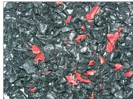
Fig. 2. PE recyclate ( $\text{PE}_{\text{rec}}$ )
