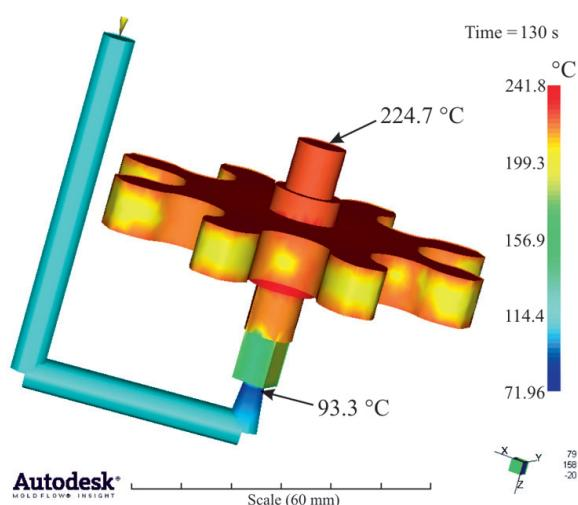
Fig. 4. Mflow simulation result presents the temperature distribution in the cast part at the moment of achieving the reaction exothermic peak (curing time 130 s) for the used resin
