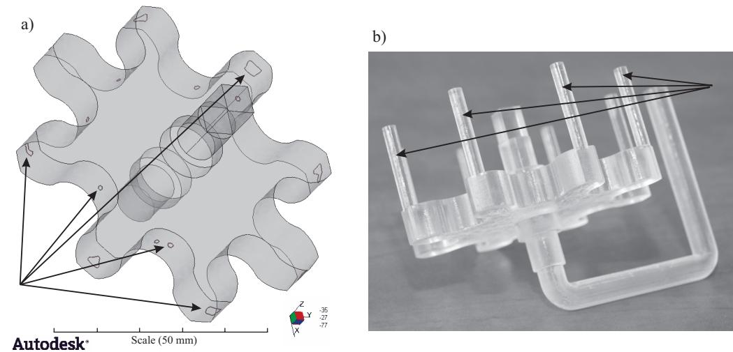
Fig. 3. Results of the mold filling simulation with air traps marked by arrows (a) and view of the master model made with stereolithographic method of adjusted shape, taking into account the results of the simulation with visible venting channels (arrows) and the runner (b)
