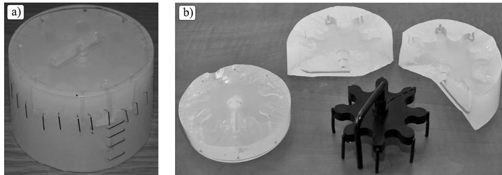
Fig. 5. Gear wheel prototype manufacturing: a) closed silicone mold, b) cast prototype made of UP composition removed from the mold and open silicone mold visible beside
