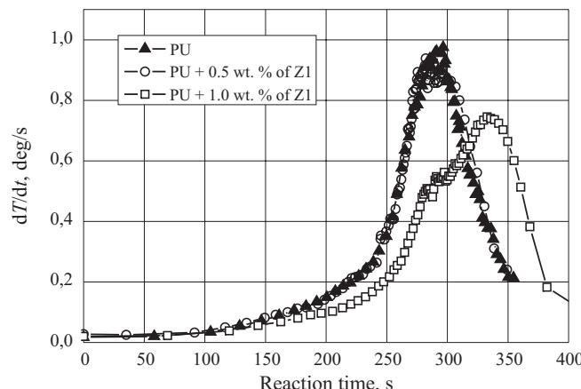
Fig. 1. Influence of Nanobent Z1 addition (0.5 or 1.0 wt. %) on differentiated gelation curves of UP composition
