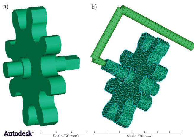
Fig. 2. Gear wheel model imported to Mflow system: a) STL model, b) FEM model with runner system
