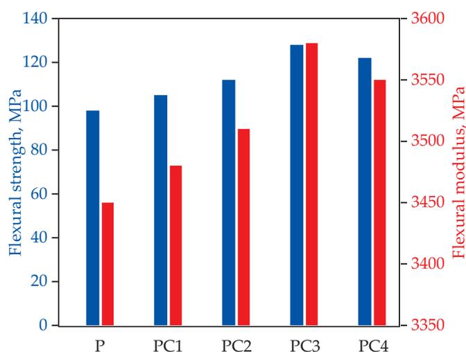
Fig. 3. Flexural strength and modulus of PLA biocomposites
