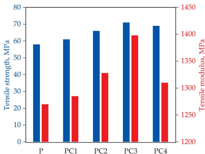
Fig. 2. Tensile strength and modulus of PLA biocomposites
