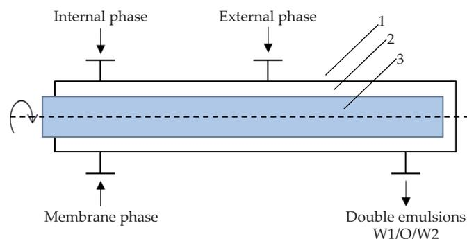
**Fig. 2.** A helicoidal (CTF) contactor for preparation of double emulsions: 1 – fixed external cylinder, 2 – annular gap, 3 – rotary cylinder
