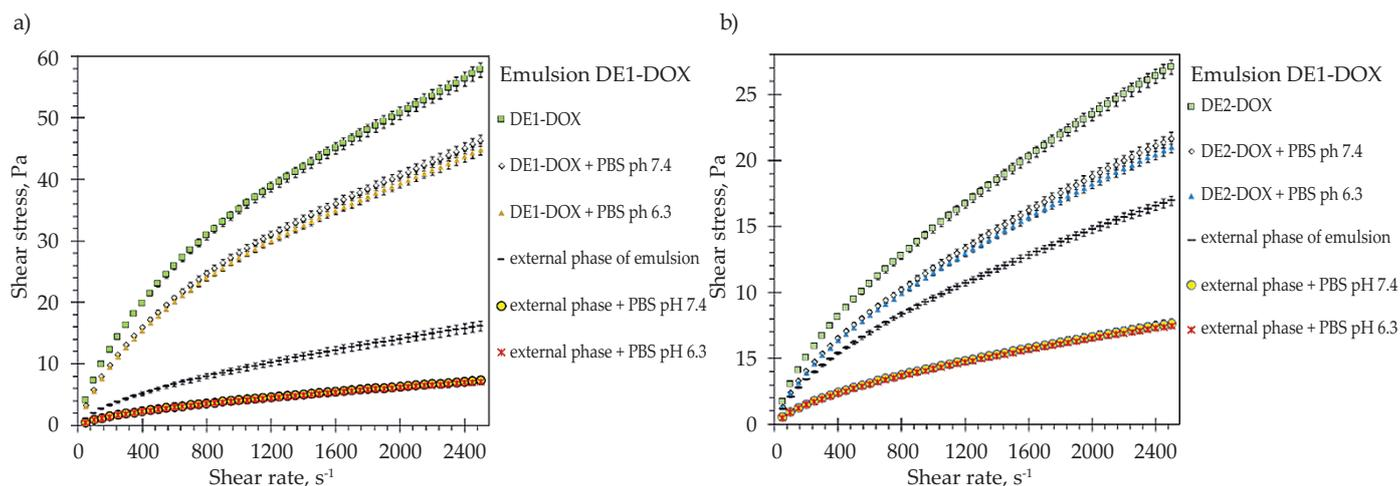
Fig. 5. The rheological curves for pH-responsive emulsions with doxorubicin and for their external phases at differing pH values
