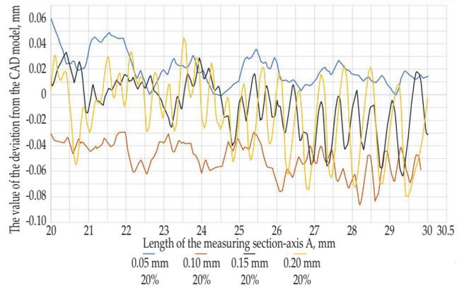
Fig. 5. Graph of the deviation value from the CAD model on the section profile of the rotor core
