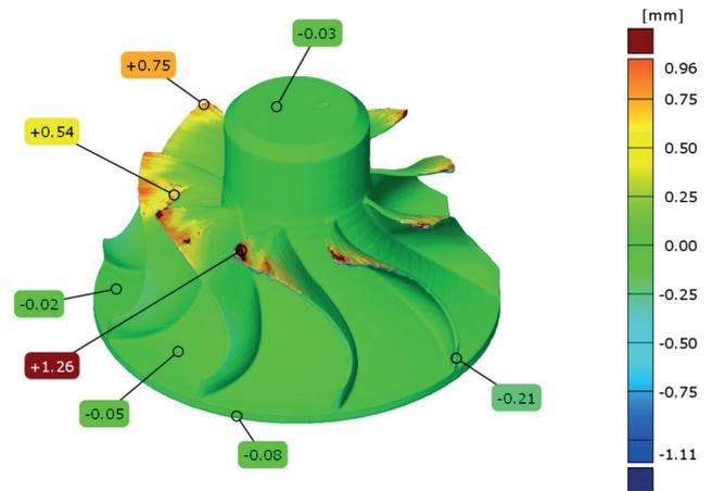
Fig. 2. Comparison of the print surface with a 0.1 mm high layer in relation to the CAD model
