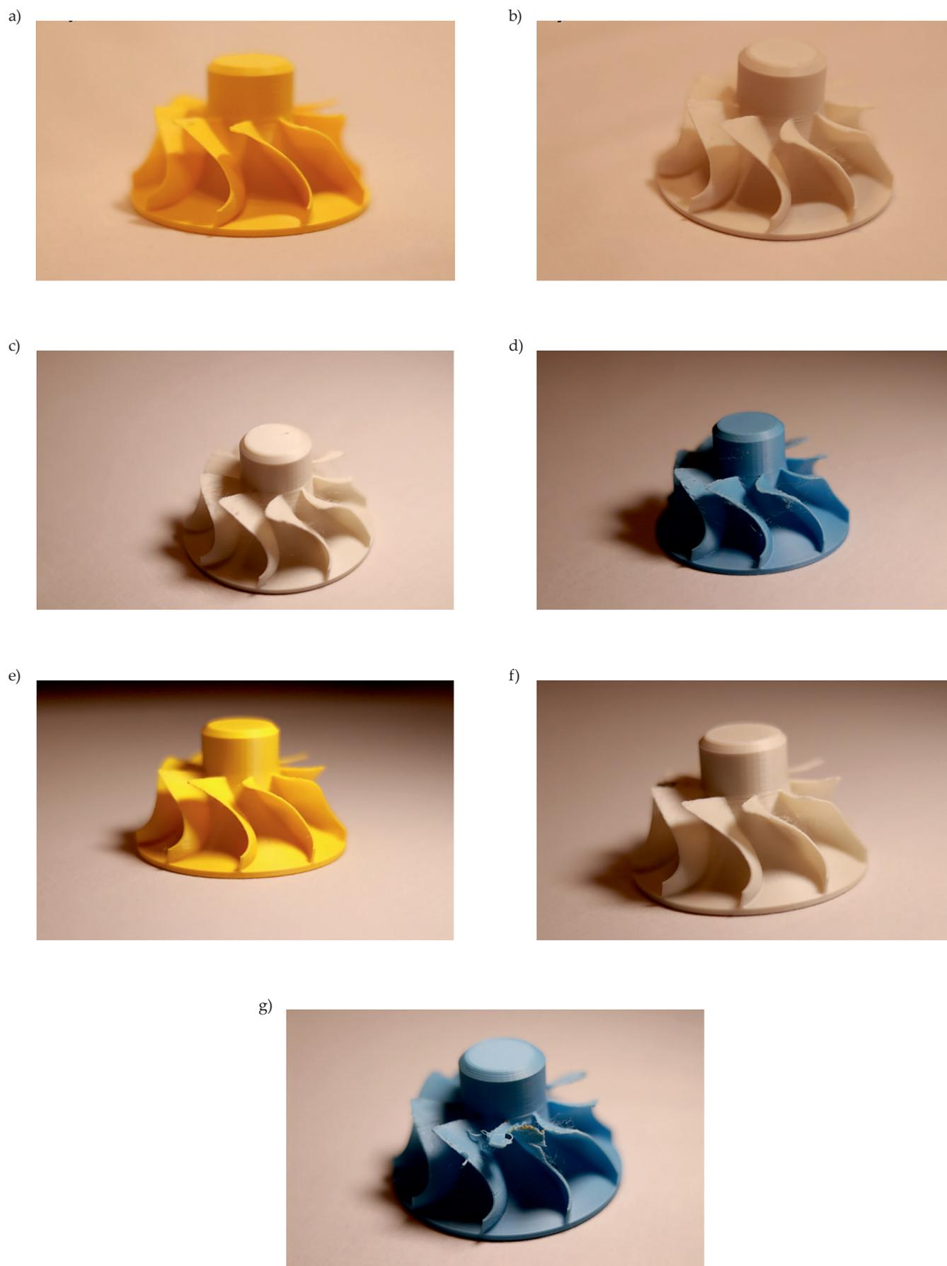
**Fig. 1.** Research models of a polymer compressor rotor produced with the use of additive techniques: a) 0.2 mm/20%, b) 0.15 mm/20%, c) 0.1 mm/20%, d) 0.05 mm/20%, e) 0.1/40%, f) 0.1/70%, g) 0.1/100%
