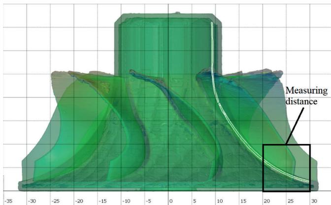
Fig. 4. Profile of the cross-section of the rotor core with the marked measurement section
