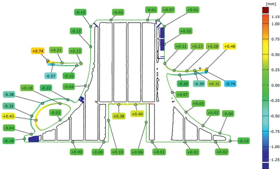
Fig. 3. Inspection cross-section in the XZ plane on a printout with a 0.05 mm high layer
