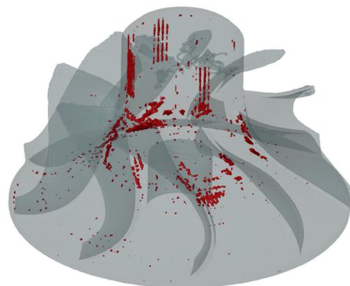
Fig. 7. Internal defects in the form of air voids on a model made with a 0.1 mm high layer and a filling density of 100%
