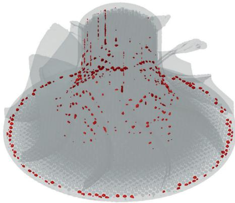
Fig. 8. Internal defects in the form of air voids on a model made with a 0.1 mm high layer and a filling density of 70%
