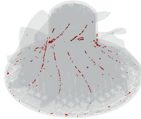
Fig. 9. Internal defects in the form of air voids on a model made with a 0.2 mm high layer and a filling density of 20%
