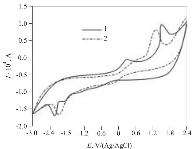
Fig. 7. Cyclic voltammograms of 4-HPEAP (1) and P-4-HPEAP (2) (cyclic voltammograms measured vs. Ag/AgCl)
