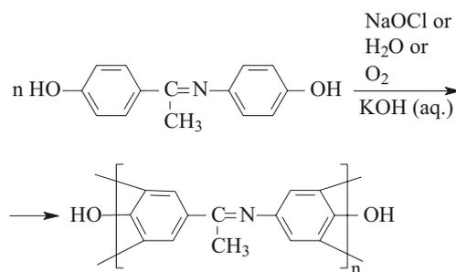
Scheme B. Synthesis of poly-4-[1-(4-hydroxyphenyl)ethylideneamino]phenol
