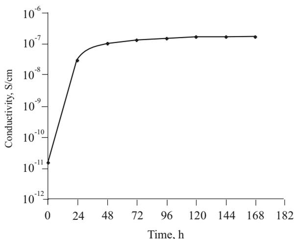
Fig. 9. Electrical conductivity of  $I_2$ -doped P-4-HPEAP vs. doping time at 25 °C
