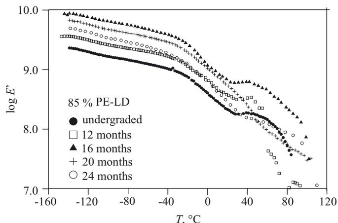
Fig. 1. Storage modulus ( $E'$ ) of 85 % PE-LD blend at 1 Hz of frequency after different exposure time
