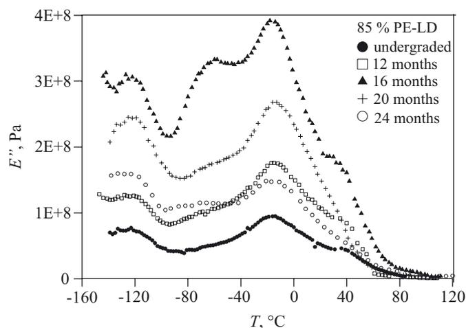
Fig. 3. Loss modulus ( $E''$ ) of 85 % PE-LD blend at 1 Hz of frequency after different exposure time
