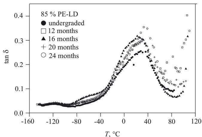
Fig. 2. Loss ( $\tan\delta$ ) of 85 % PE-LD blend at 1 Hz of frequency after different exposure time
