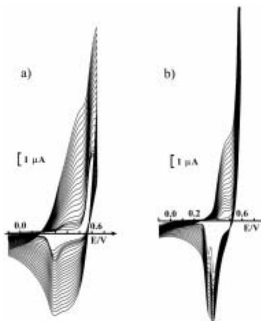
Fig. 6. Cyclic voltammograms recorded during electropolymerization of 5 mM solution of M2 in: a) 0.2 M  $(\text{Bu})_4\text{NPF}_6/\text{CH}_3\text{CN}$ , b) 0.2 M  $(\text{Bu})_4\text{NPF}_6/\text{CH}_2\text{Cl}_2$ ; scan rate 0.02 V/s
