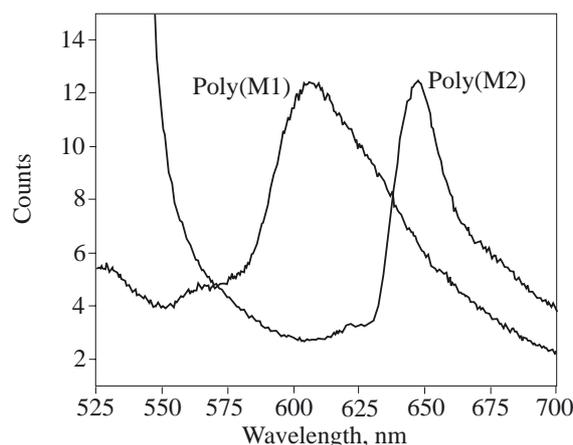
Fig. 11. Photoluminescence spectra of poly(M1) and poly(M2) solid in an air; films of about 50 nm thick were deposited electrochemically on optically transparent ITO
