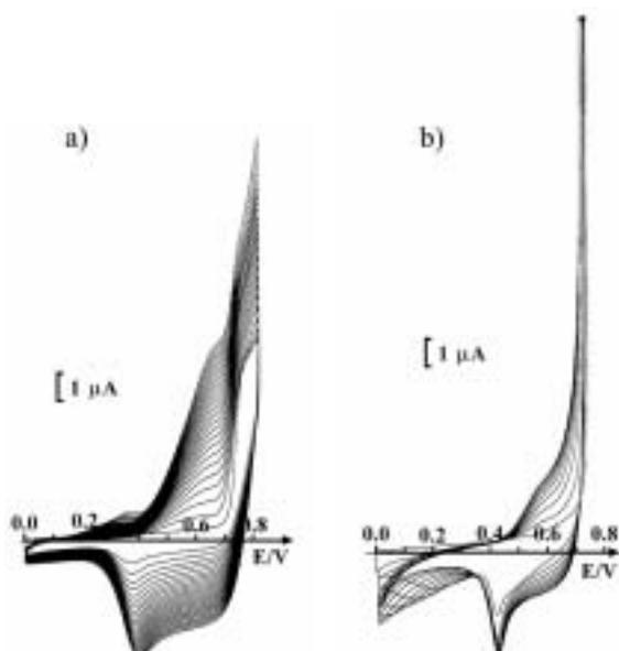
Fig. 5. Cyclic voltammograms recorded during electropolymerization of 5 mM solution of M1 in: a) 0.2 M  $(\text{Bu})_4\text{NPF}_6/\text{CH}_3\text{CN}$ , b) 0.2 M  $(\text{Bu})_4\text{NPF}_6/\text{CH}_2\text{Cl}_2$ ; scan rate 0.02 V/s
