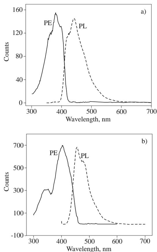
Fig. 2. Photoluminescence (PL) and photoexcitation (PE) spectra of  $\sim 0.5\text{ mM}$  solutions in  $\text{CH}_2\text{Cl}_2$  of: a) M1, b) M2
