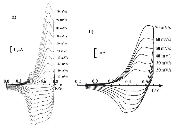
Fig. 8. Cyclic voltammetry curves recorded at variable scan rates in  $\text{CH}_3\text{CN}$  solution containing 0.2 M of  $(\text{Bu})_4\text{NPF}_6$  for solid films of: a) poly(M1), b) poly(M2); scan rate 0.05 V/s
