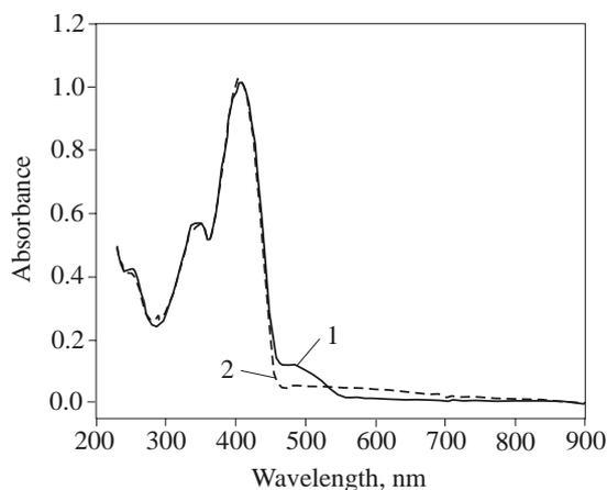
Fig. 7. UV-Vis absorption spectra of M2 solution in  $\text{CH}_2\text{Cl}_2$  measured before (curve 1) and after electropolymerization (curve 2)
