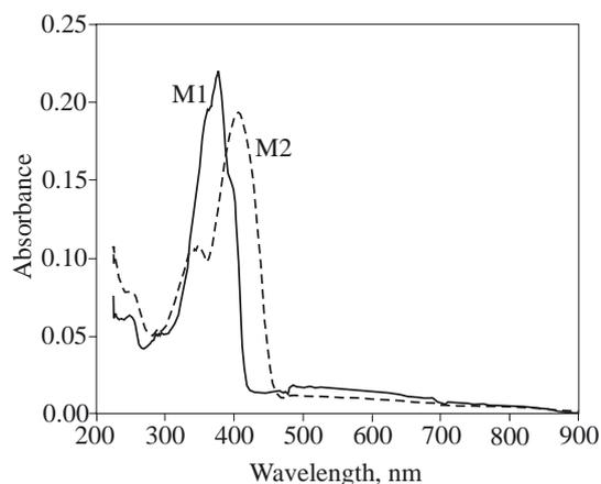
Fig. 1. UV-Vis absorption spectra of  $\sim 0.5\text{ mM}$  solutions in  $\text{CH}_2\text{Cl}_2$  of: M1 — solid line, M2 — dashed line
