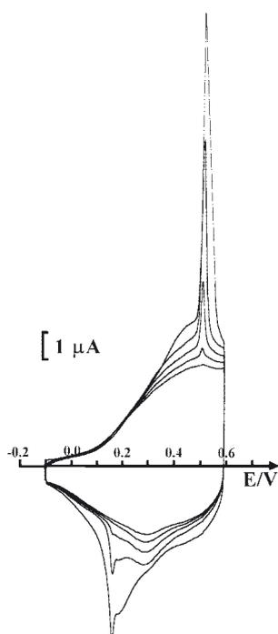
Fig. 9. Cyclic voltammograms recorded in  $\text{CH}_3\text{CN}$  solution containing 0.2 M of  $(\text{Bu})_4\text{NPF}_6$  for solid film of poly(M2) that was synthesized in  $\text{CH}_2\text{Cl}_2$  solution; scan rate 0.05 V/s
