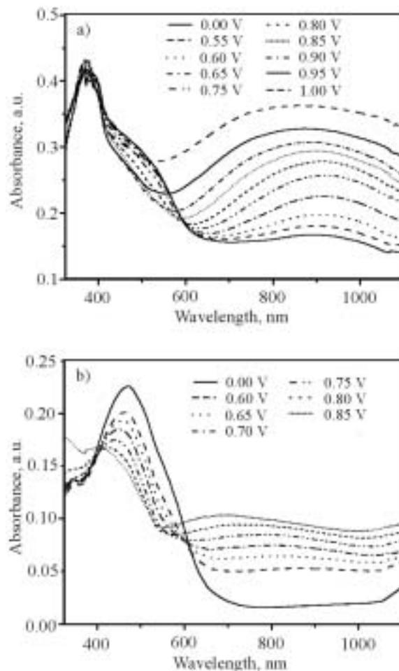
Fig. 10. UV-Vis spectroelectrochemistry of polymer solid films on optically transparent ITO electrodes in  $\text{CH}_3\text{CN}$  solution containing 0.2 M  $(\text{Bu})_4\text{NPF}_6$ : a) poly(M1), b) poly(M2); each spectrum recorded at potential indicated in the insert of the figure
