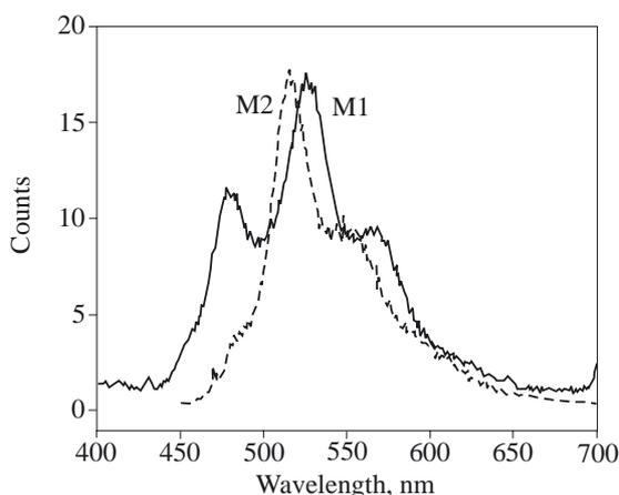
Fig. 3. Solid state PE spectra of M1 and M2, taken in an air; thin films were cast on microscopic glass slides from  $\text{CH}_2\text{Cl}_2$  solutions
