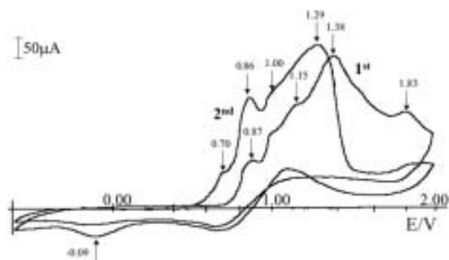
Fig. 4. Cyclic voltammetry curves on Pt electrode for  $\sim 1$  mM solution of M2 in 0.2 M  $(\text{Bu})_4\text{NPF}_6/\text{CH}_3\text{CN}$ ; 1 — first scan, 2 — second scan, both scans at 0.1 V/s
