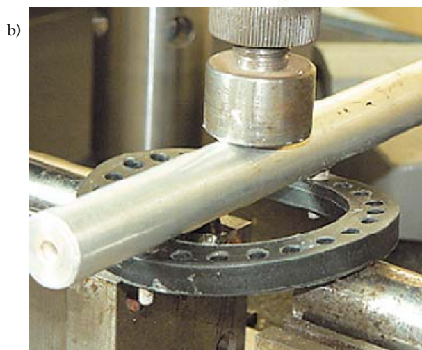
Fig. 3. Configuration of the bending tests (a) and moment of testing (b)
