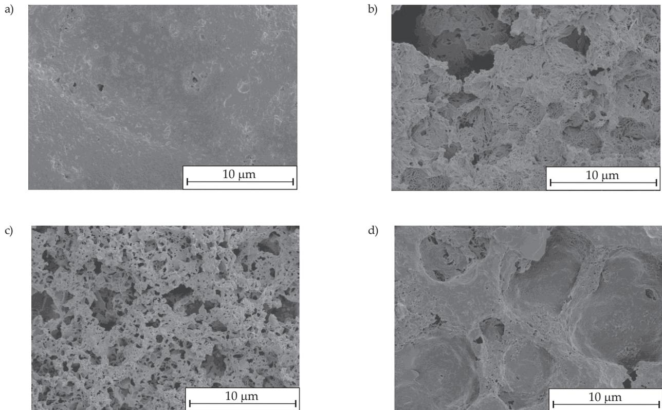
Fig. 7. SEM images of PLA samples subjected to degradation in proteinase K for 7 weeks: a) PLA\_PK, b) PLA+C+E\_PK, c) PLA+T+E\_PK, d) PLA+T+C\_PK
