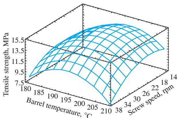
Fig. 2. Response surface plot of tensile strength
