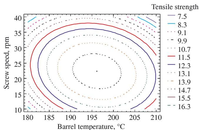
Fig. 1. Contour plot of tensile strength (in MPa) dependent on barrel temperature and screw speed
