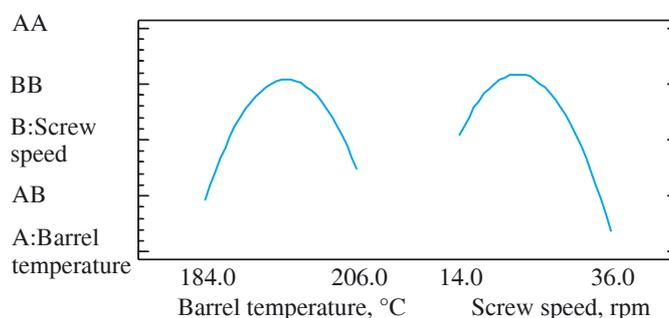
Fig. 4. Main effect plot of tensile strength
