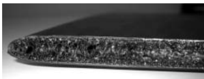
Fig. 10. Example of microcellular PP panel, produced by MuCell precision opening (according to [56], changed)
