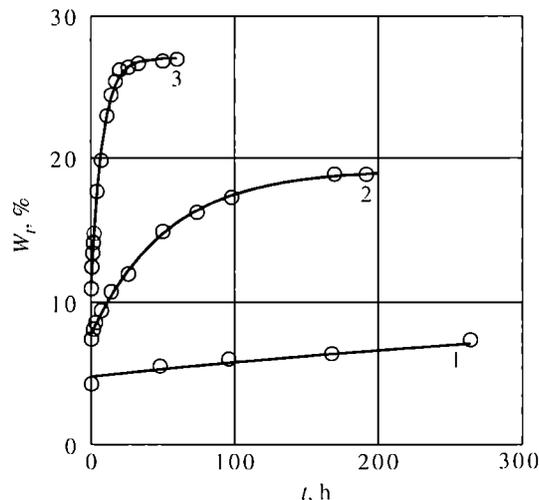
Fig. 1. The effects of time ( $t$ ) and starch content ( $S$ ) on water absorption by biodegradable samples: 1 —  $S = 20$  %, 2 —  $S = 33$  %, 3 —  $S = 47$  %;  $T = 20$  °C
