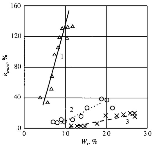
Fig. 3. The relationship between breaking strain ( $\epsilon_{max}$ ) and water content ( $W_t$ ) of the materials with different  $S$  levels. Descriptions of curves as in Fig. 1
