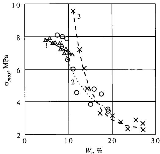
Fig. 2. The relationship between breaking stress ( $\sigma_{max}$ ) and water content ( $W_t$ ) of the materials with different  $S$  levels. Descriptions of curves as in Fig. 1
