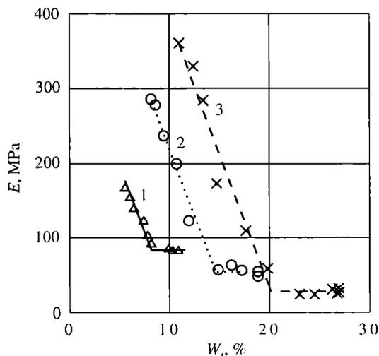
Fig. 4. The effects of moisture content ( $W$ ) and starch content  $S$  in a composition on elasticity modulus ( $E$ ): 1 —  $S = 20 \%$ , 2 —  $S = 33 \%$ , 3 —  $S = 47 \%$ ;  $E_m$  — minimum value of elasticity modulus
