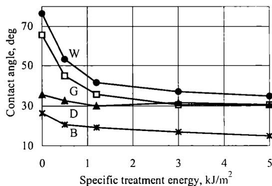
Fig. 1. Influence of specific treatment energy on the contact angle of non-treated GPPS; liquids: W — twice distilled water, G — glycerol, D — diiodomethane, B —  $\alpha$ -bromonaphthalene
