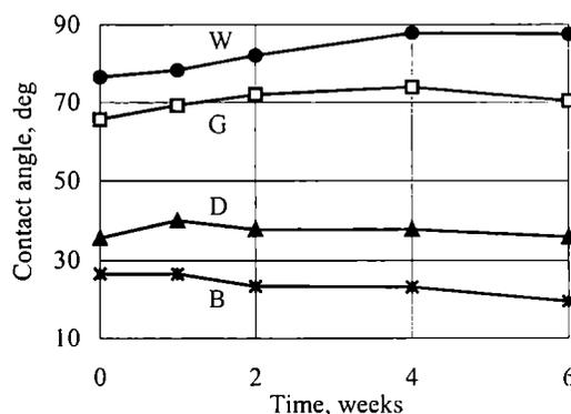
Fig. 2. Influence of storage time on the contact angle of GPPS film (explanations as in Fig. 1)
