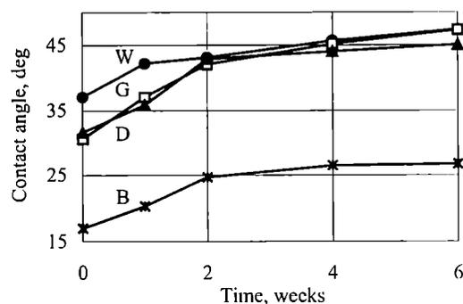
Fig. 5. Influence of storage time on the contact angle of GPPS film treated with  $E_j = 3.0$   $\text{kJ}/\text{m}^2$  (explanations as in Fig. 1)
