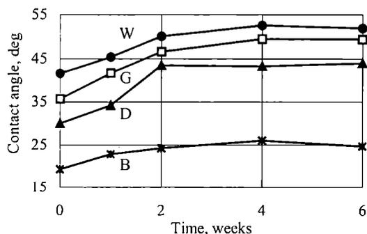
Fig. 4. Influence of storage time on the contact angle of GPPS film treated with  $E_j = 1.2$   $\text{kJ}/\text{m}^2$  (explanations as in Fig. 1)
