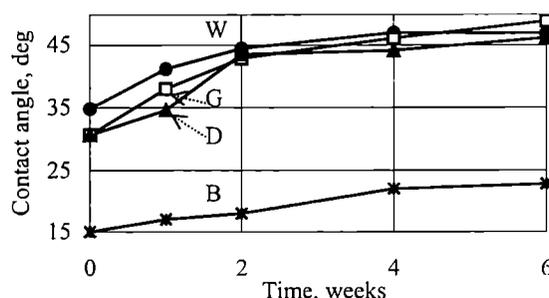
Fig. 6. Influence of storage time on the contact angle of GPPS film treated with  $E_j = 5.0$   $\text{kJ}/\text{m}^2$  (explanations as in Fig. 1)
