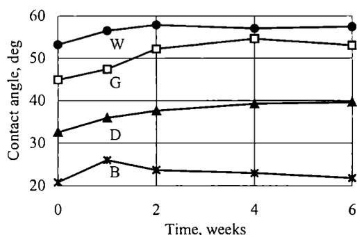
Fig. 3. Influence of storage time on the contact angle of GPPS film treated with  $E_j = 0.5$   $\text{kJ}/\text{m}^2$  (explanations as in Fig. 1)
