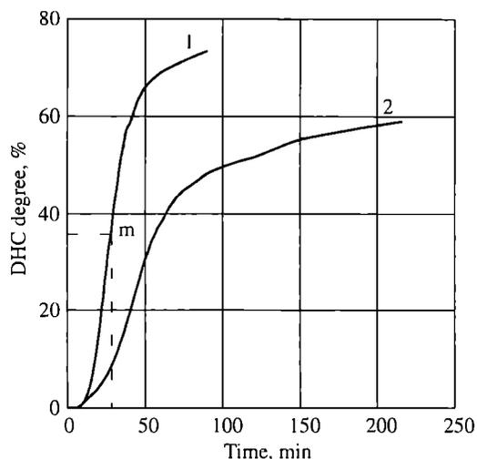
Fig. 1. Comparison of DHC curves of PVC (1) and its mixture with 12.6 wt.% of PE (2) dehydrochlorination at temp. 240°C; m — maximal DHC rate
