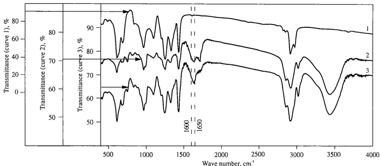
Fig. 5. FT-IR diagram of PVC and its carbonization products showing different DHC degrees: 1 — PVC, 2 — carbonization product, 21% DHC degree, 3 — carbonization product, 58% DHC degree
