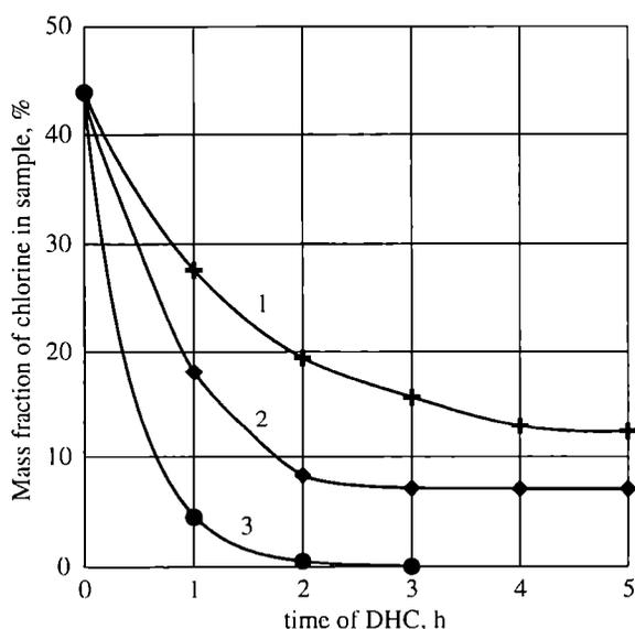
Fig. 2. Effect of temperature on PVC window profiles dehydrochlorination; temperature: 1 — 260°C, 2 — 300°C, 3 — 400°C
