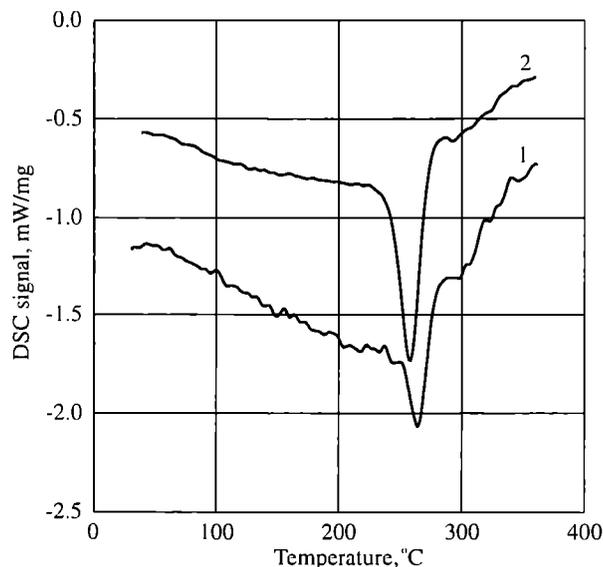
Fig. 4. DSC curves of PVC samples with different densities: 1 — powdered PVC, 2 — PVC pellet formed under pressure 1.4 MPa; heating rate  $2^\circ\text{C}/\text{min}$
