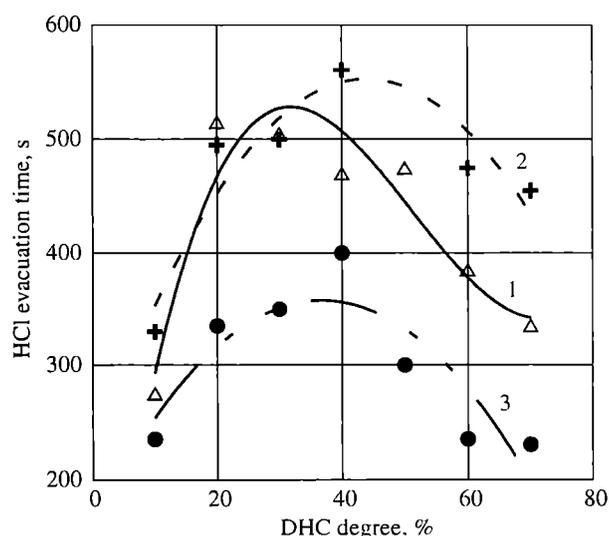
Fig. 3. Effects of DHC degree and temperature on time of HCl evacuation from PVC sample at various temperatures; temperature: 1 — 240°C, 2 — 250°C, 3 — 260°C (with higher inert gas velocity)
