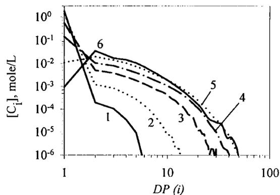
Fig. 2. Concentrations of cyclics ( $[C_i]$ ) obtained by Monte Carlo simulations of reshuffling in  $\epsilon$ -caprolactone polymerization computed for the same conditions as in Fig. 1. Different curves correspond to different degrees of monomer conversions — description as in Fig. 1
