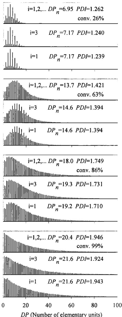
Fig. 9. MWD plots of the products of composite monomer ( $C_2$ ) polymerizations proceeding with a reshuffling of segmental exchange and cyclization leading to  $C_i$  obtained by Monte Carlo simulations ( $[C_2]_0 = 1.0$ ,  $[I]_0 = 0.1$ ,  $k_{p2}/k_{tr} = 10^1$ ,  $k_{p2}[C_2]_0/\Sigma k_{ci} = 10^2$ ,  $\Sigma[C_i]_e = 10^{-3}$ )
