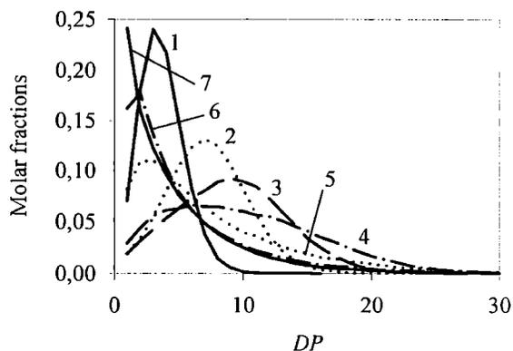
Fig. 3. Frequency distribution plots obtained by Monte Carlo simulations of reshuffling in  $\epsilon$ -caprolactone polymerization computed for conditions similar to those in Fig. 1 but  $[M]_0 = 0.2$  mol/L. Different curves correspond to different degrees of monomer conversions: 1 — 12.5%, 2 — 32.5%, 3 — 48.3%, 4 — 73.1%, 5 — 92.5%, 6 — 97.8%, 7 — 99.7% (close to the equilibrium value)
