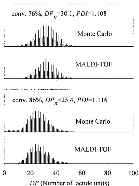
Fig. 10. *MWD* of the products of composite monomer ( $C_2$ ) polymerizations (proceeding with a reshuffling of segmental exchange and cyclization leading to  $C_3$  obtained by Monte Carlo simulations) fitted to the observed (MALDI-TOF) [9] relative concentrations of oligomers in *L,L*-dilactide polymerization ( $k_p/k_w = 83.3$ ,  $k_{c3}/k_{tr} = 1.07 \cdot 10^{-3} \text{ mol/L} \approx [C_3]_e$ )
