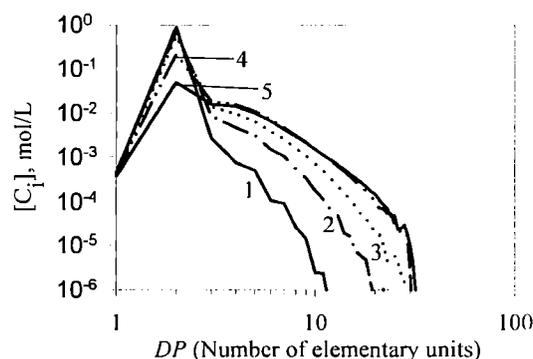
Fig. 12. Concentrations of cyclics ( $[C_i]$ ) obtained by Monte Carlo simulations of reshuffling in  $\epsilon$ -caprolactone dimer polymerization computed for the same conditions as in Fig. 11. Different plots correspond to different degrees of  $C_2$  conversion — descriptions as in Fig. 11
