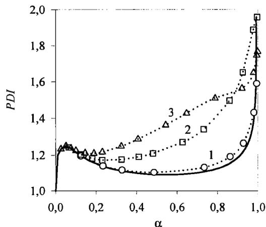
Fig. 7. Polydispersity index (PDI) versus monomer conversion ( $\alpha$ ) plotted for simulations presented in Figs. 1, 3, and 5 beside a curve (solid line) computed for the identical polymerization process with reshuffling but without cyclization (initial monomer concentrations do not matter);  $[M]_0$  in mol/L: 1 — 2, 2 — 0.2, 3 — 0.08
