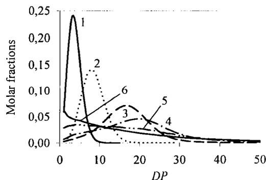
Fig. 1. Frequency distribution plots obtained by Monte Carlo simulations of reshuffling in  $\epsilon$ -caprolactone polymerization computed for conditions:  $[M]_0/[I]_0 = 22.7$ ,  $[M]_0 = 2$  mol/L, rate constant determined by the authors of ref. [5] for 20 °C. Different curves correspond to different degrees of monomer conversion: 1 — 12.5%, 2 — 33.0%, 3 — 73.4%, 4 — 93.0%, 5 — 99.5%, 6 — 99.95% (close to the equilibrium value)
