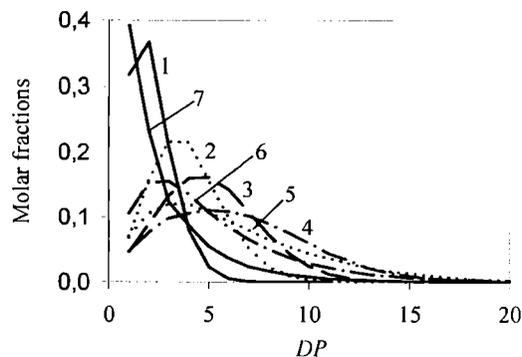
Fig. 5. Frequency distribution plots obtained by Monte Carlo simulations of reshuffling in  $\epsilon$ -caprolactone polymerization computed for conditions similar to those in Fig. 1 but  $[M]_0 = 0.08$  mol/L. Different curves correspond to different degrees of monomer conversions: 1 — 5.1%, 2 — 14.5%, 3 — 23.0%, 4 — 40.6%, 5 — 64.6%, 6 — 78.8%, 7 — 99.9% (close to the equilibrium value)
