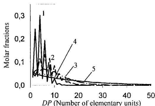
Fig. 11. Frequency distribution plots obtained by Monte Carlo simulations of reshuffling in  $\epsilon$ -caprolactone dimer polymerization computed for conditions similar to those in Fig. 1 but  $[C_2]_0 = 1 \text{ mol/L}$  ( $2[C_2]_0/[I]_0 = 22.7$  and rate constant the same as in Fig. 1). Different plots correspond to different degrees of  $C_2$  conversion: 1 — 12%, 2 — 28%, 3 — 46%, 4 — 78%, 5 — 95% (equilibrium value)
