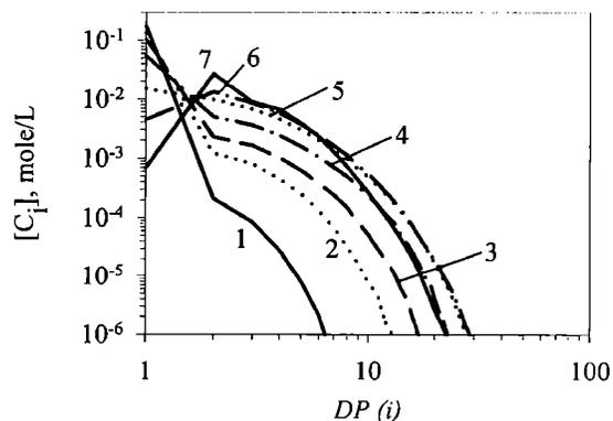
Fig. 4. Concentrations of cyclics ( $[C_i]$ ) obtained by Monte Carlo simulations of reshuffling in  $\epsilon$ -caprolactone polymerization computed for the same conditions as in Fig. 3. Different curves correspond to different degrees of monomer conversions — description as in Fig. 3
