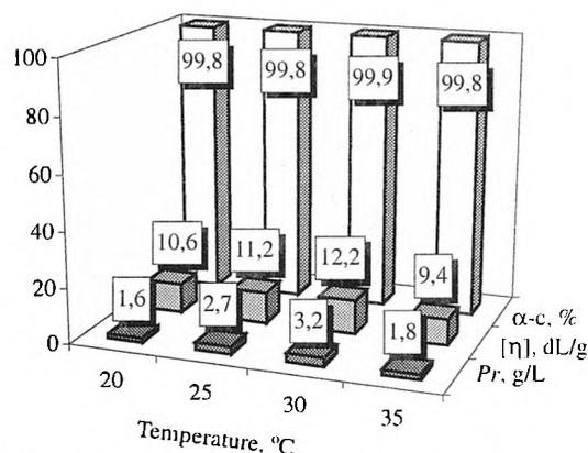
**Fig. 1.** Effect of biosynthesis temperature on cellulose productivity (Pr),  $\alpha$ -cellulose content ( $\alpha$ -c) and intrinsic viscosity ( $[\eta]$ )
