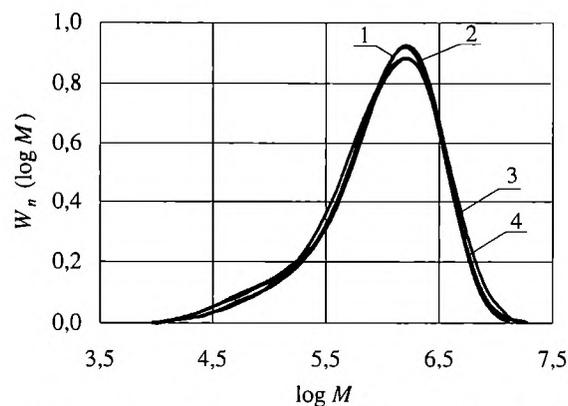
Fig. 4. Effect of medium pH on molecular weight distribution of bacterial cellulose; pH: 1 — 3.8; 2 — 4.8; 3 — 6.0; 4 — 7.5 ( $W_n$  — see Fig. 2)
