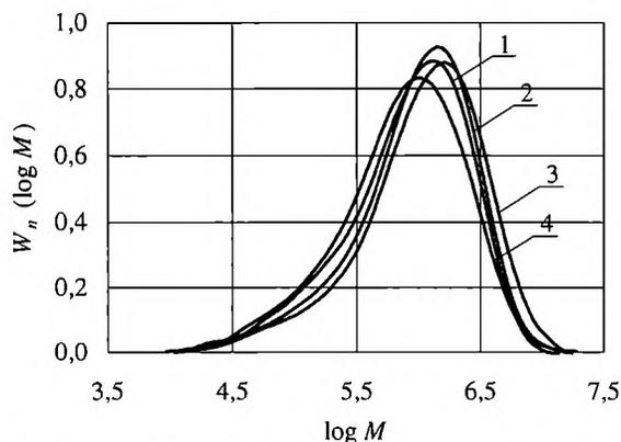
Fig. 2. Effect of biosynthesis temperature on molecular weight distribution of bacterial cellulose; temperature 1 — 20 °C, 2 — 25 °C, 3 — 30 °C, 4 — 35 °C ( $W_n$  — share of the given  $M$  value)
