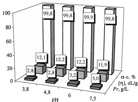
Fig. 3. Effect of medium pH on cellulose productivity ( $Pr$ ),  $\alpha$ -cellulose content ( $\alpha$ -c) and intrinsic viscosity ( $[\eta]$ )
