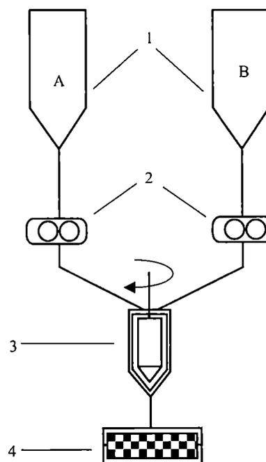
Fig. 1. The reaction injection molding process of PUR: 1 — component A (polyetherdiol or polyesterdiol + diol + additives) and component B (diisocyanate or oligomer with isocyanate end-groups), 2 — high pressure pump, 3 — mixing head, 4 — mold with reacting PUR mixture
