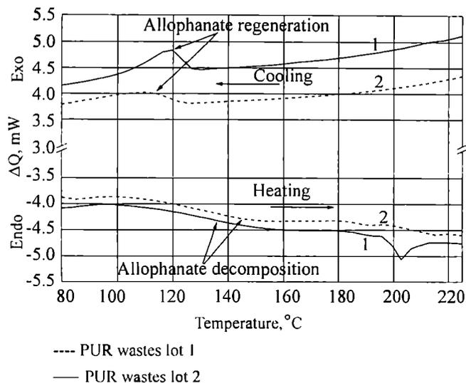
Fig. 3. DSC of PUR foams wastes: 1 — sample first, 2 — sample second; heating and cooling rate — 10 deg/min
