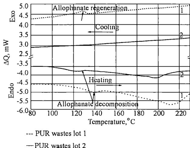
Fig. 4. DSC of PUR foams wastes after reactive extrusion: 1 — PUR foams wastes extruded, 2 — PUR foams wastes coextruded with 10 wt. % of unplasticized PVC (PVC-U); heating and cooling rate — 10 deg/min
