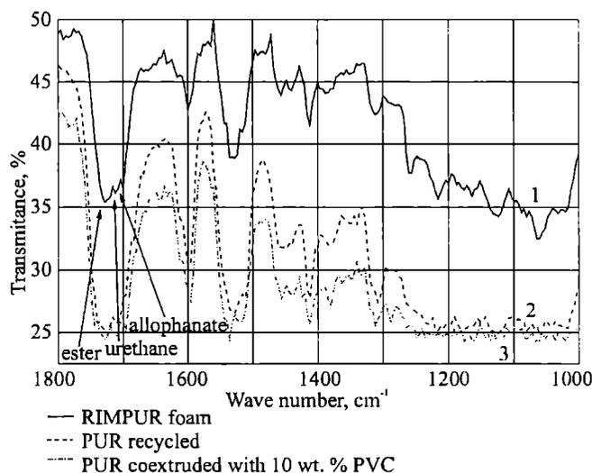
Fig. 5. IR spectra of original PUR foam wastes (1), its recycled blend (2) and recycled blend coextruded with 10 wt. % of PVC-U (3)
