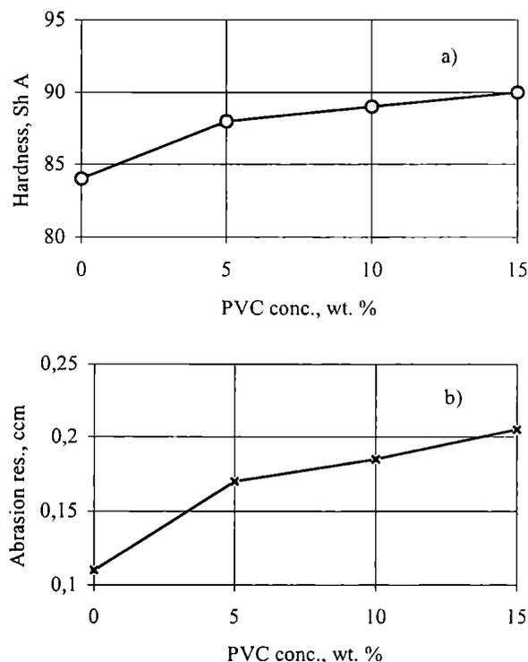
**Fig. 7. Hardness (a) and abrasion (b) vs. PVC-U concentration in the recycled PUR foams wastes**
