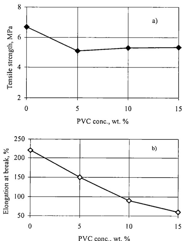
**Fig. 6. Tensile strength (a) and elongation at break (b) vs. PVC-U concentration in the recycled PUR foams wastes**
