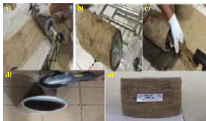
Fig. 3. a) Wet and wrapped kenaf mat around the mold, b) sample left for a while to dry well, c) sample extracted from the mandrel, d) finishing the sample, e) hardened kenaf mat composite elliptical tube
