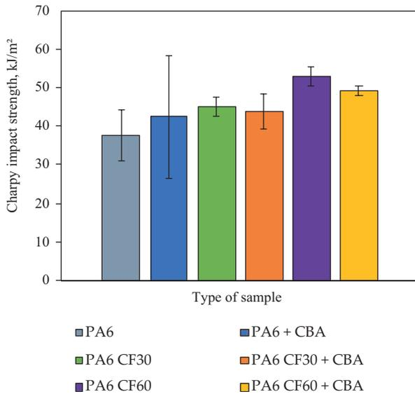
Fig. 7. Average impact strength of the tested PA6 composites with the standard deviation
