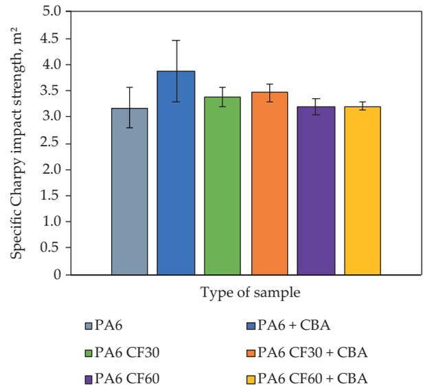
Fig. 8. Average specific impact strength of the tested PA6 composites with the standard deviation
