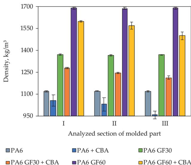
Fig. 2. The average density of the tested polyamide composites along with the standard deviation in individual zones along the flow path
