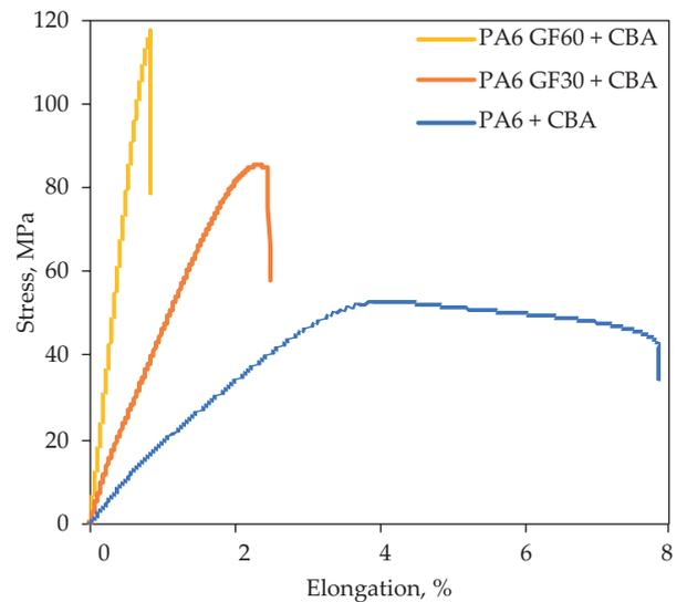
Fig. 5. The relationship between the stress and the elongation of samples
