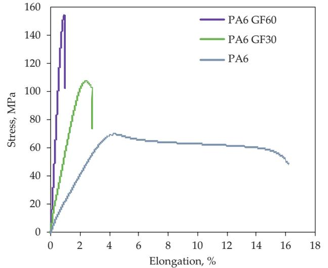
Fig. 4. The relationship between the stress and the elongation of samples
