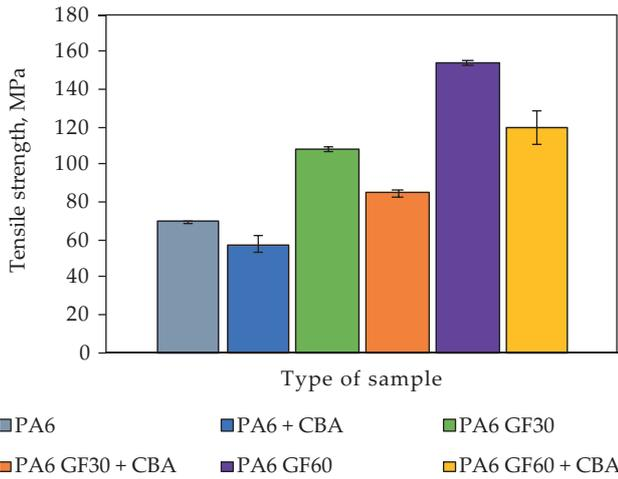
Fig. 3. Average tensile strength of the series tested, together with the standard deviation
