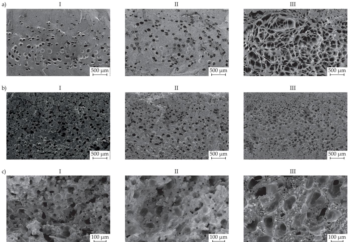
Fig. 11. The core structure of the tested moldings in individual zones: a) PA6 + CBA, b) PA6 GF30 + CBA, c) PA6 GF60 + CBA; I – beginning, II – middle, III – end of the measuring section
