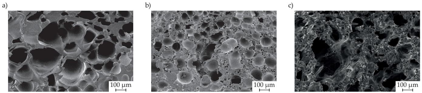
Fig. 10. The core structure of the molded part in zone III: a) PA6 + CBA, b) PA6 GF30 + CBA, c) PA6 GF60 + CBA
