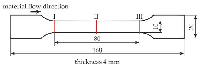
Fig. 1 Geometry of the test specimen - geometrical dimensions with the division of the molding into measurement zones: I – beginning, II – middle, III – end of the measuring section
