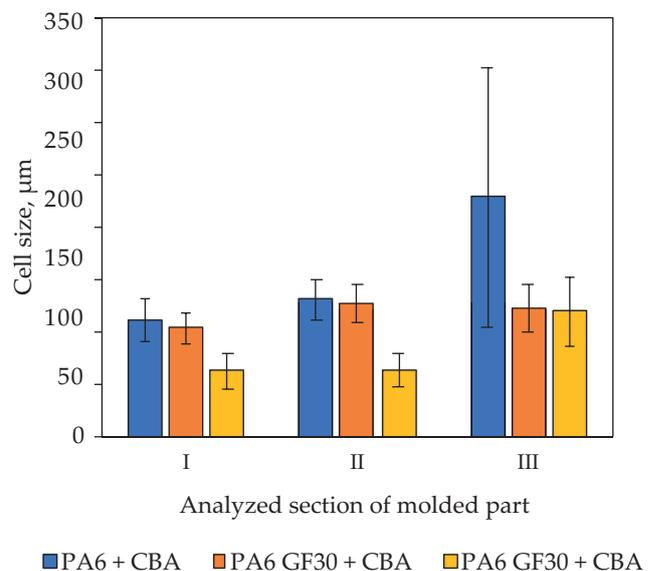
Fig. 9. The average size of the pores in the individual zones core of the tested moldings
