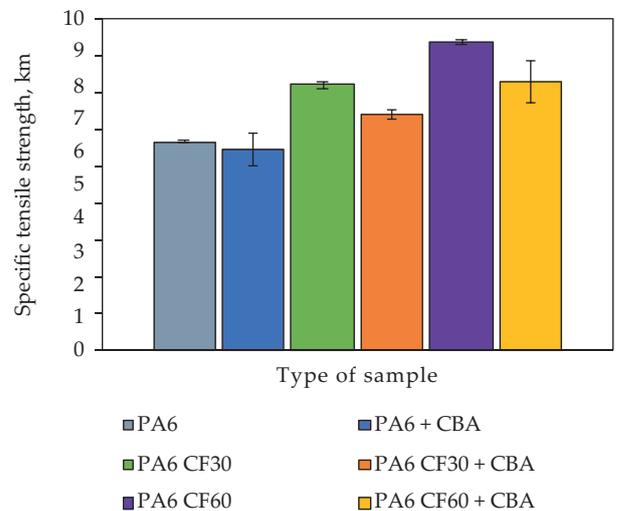
Fig. 6. Specific tensile strength of the tested series of polyamide 6
