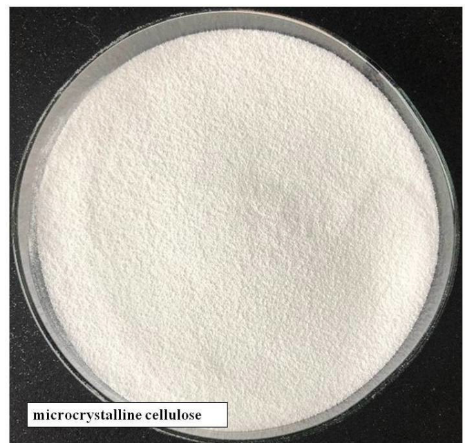
Fig. 2. Microcrystalline cellulose (Avicel PH – 101), with a diameter of 2–6 \mu\text{m} , bulk density 0.36 \text{g}/\text{cm}^3
