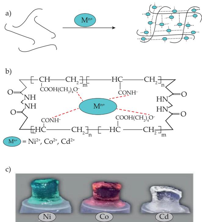
Fig. 6. The interaction between hydrogels and metals: a) and b) the proposed mechanism, c) photographs of hydrogels after heavy metals adsorption
