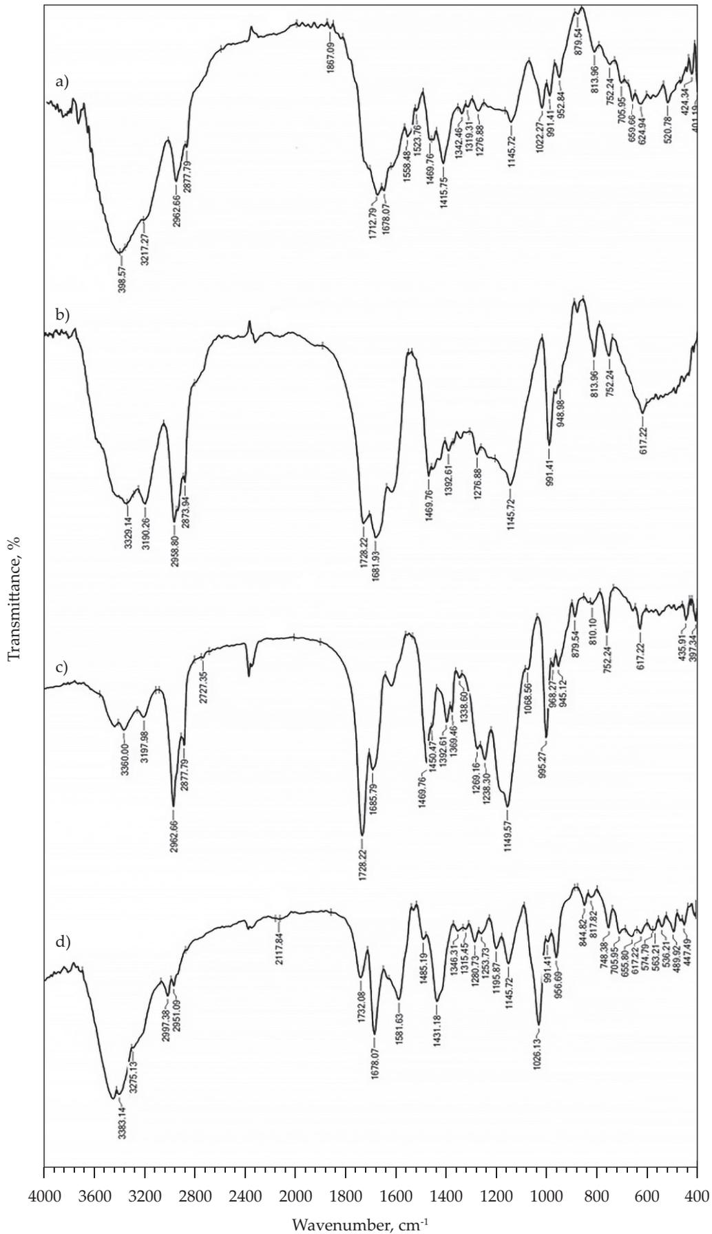
Fig. 2. FTIR spectra of: 70HBA/30AAm hydrogel before (a) and after adsorption of (b) Co<sup>2+</sup>, (c) Ni<sup>2+</sup>, and (d) Cd<sup>2+</sup>
