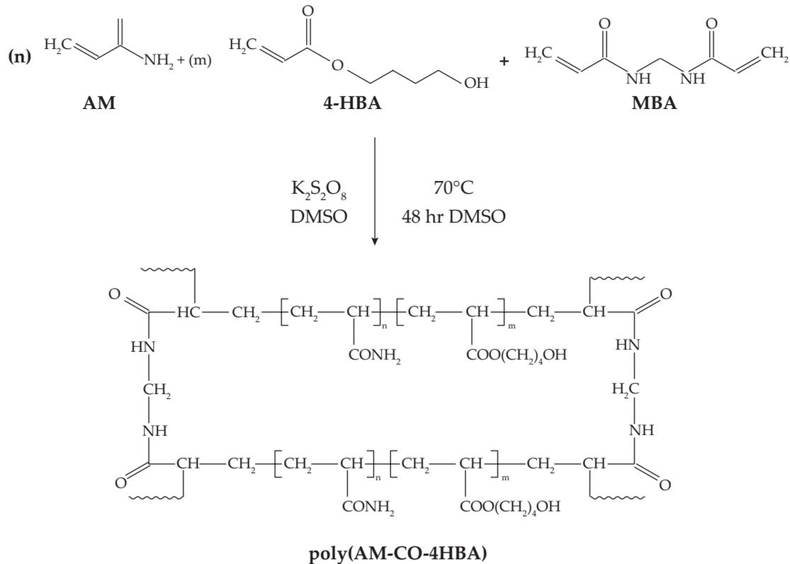
Fig. 1. Reaction scheme of poly(AM-co-4HBA) crosslinking
