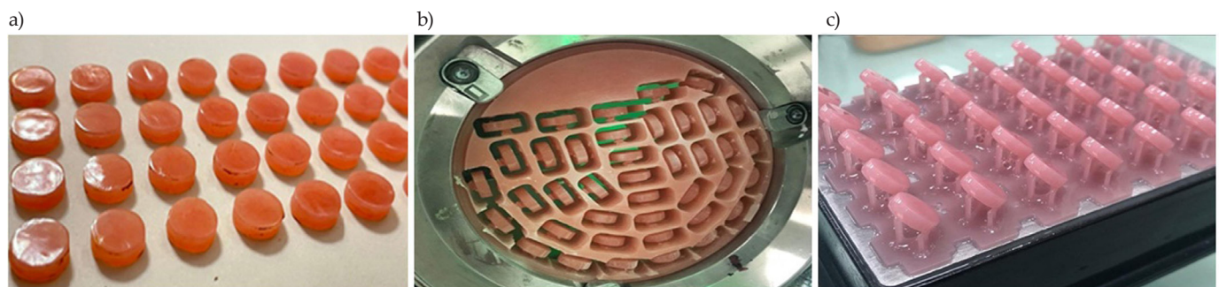
Fig. 2. Denture base material discs: a) conventional, b) milled, c) 3D-printed
