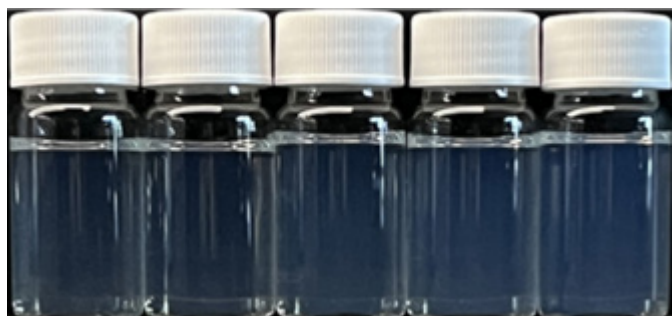
Fig. 1. Opacity of water phase based on AAPH with CC-301 colloidal silica (left 0% AAPH, right 2% AAPH)
