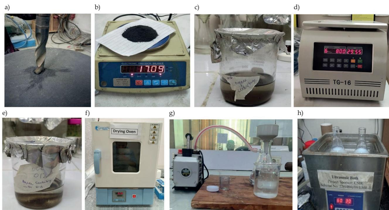
Fig. 2. GO synthesis: a) obtaining graphite flakes, b) weighing, c) before reaction, d) centrifuge, e) after centrifugation, f) dryer, g) vacuum filtration, and h) ultrasonic exfoliation
