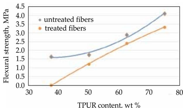
Fig. 5. Flexural strength properties of treated and untreated kenaf fiber TPUR-NR composites
