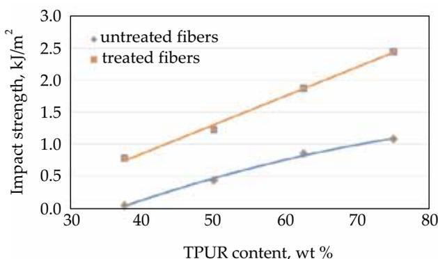
Fig. 6. Impact properties of treated and untreated kenaf fiber TPUR-NR composites
