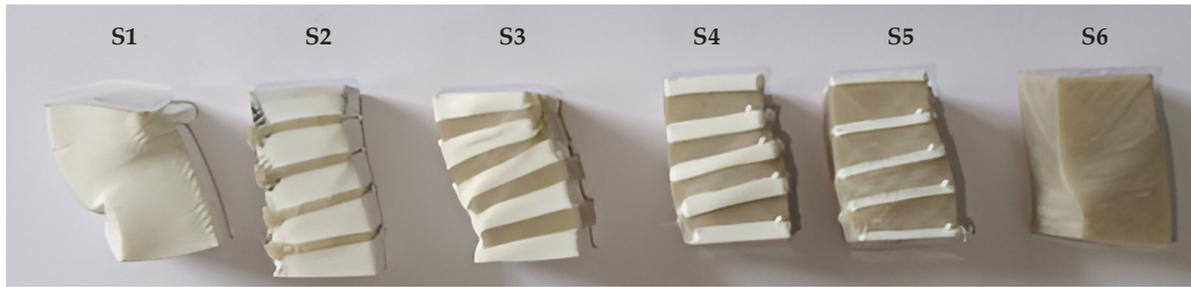
Fig. 5. The samples after compression test
