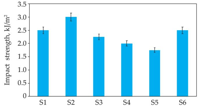
Fig. 7. Impact strength of PLA, PLA-PLA/ $\text{Al}_2\text{O}_3$  and PLA/ $\text{Al}_2\text{O}_3$
