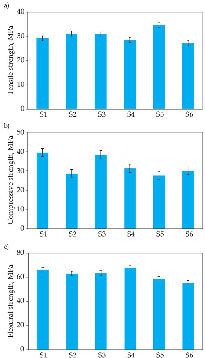
**Fig. 4. Mechanical properties: a) tensile strength, b) compressive strength, c) flexural strength**
