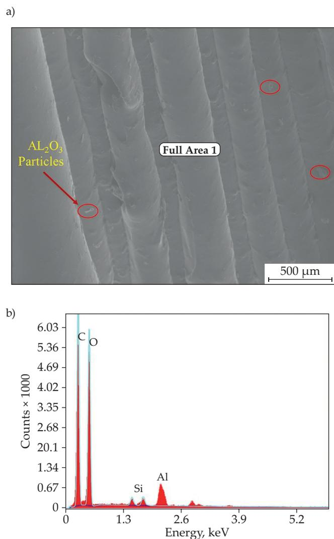
Fig. 1. FESEM images of PLA-PLA/Al<sub>2</sub>O<sub>3</sub> (a), EDX analysis (b)
