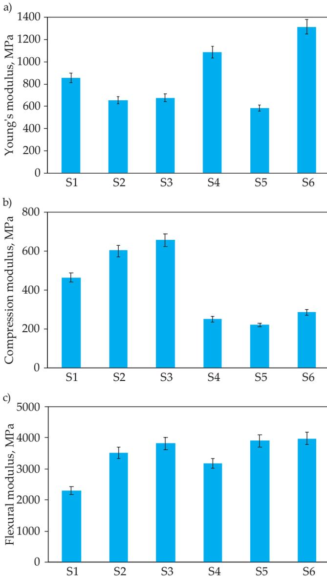
Fig. 6. Mechanical properties: a) Young's modulus, b) compression modulus, c) flexural modulus
