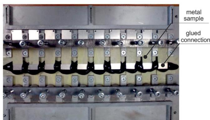
Fig. 1. Samples after bonding and pressing
