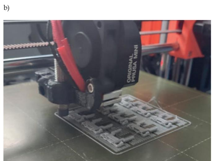
Fig. 7. Chain links cut into layers (a) and printing process using FFF technology (b)
