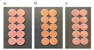
Fig. 2. Acrylic resin specimens fabricated using conventional (a), milling (b) and 3D-printing (c)
