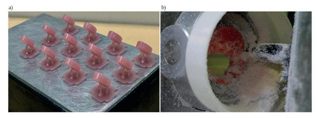
Fig. 1. a) 3D-printed acrylic resin specimens; b) CAD/CAM milling of the PMMA blanks
