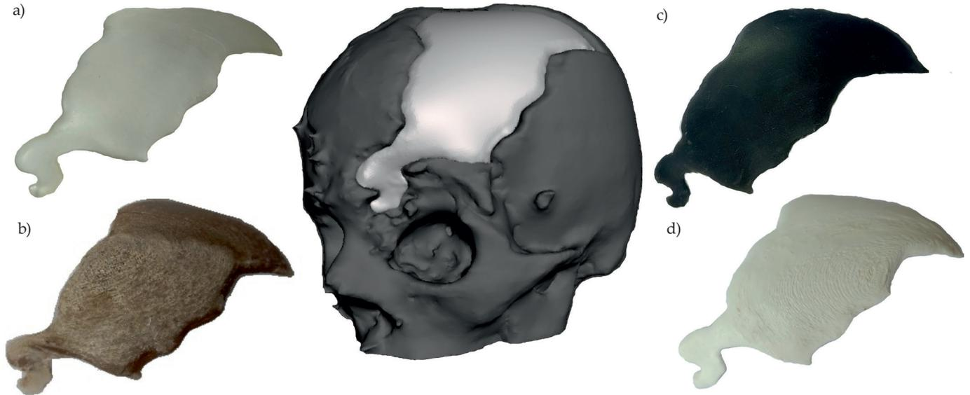
Fig. 3. 3D-CAD model of a facial defect and the implants obtained from: a) MED610, b) PEEK, c) UV resin, d) PLA
