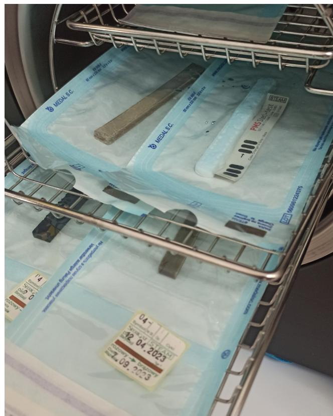
**Fig. 1.** Autoclave chamber containing packed and sterilized samples
