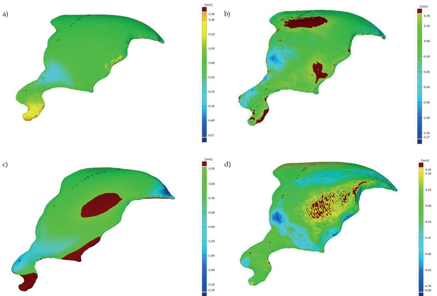
Fig. 4. 3D maps of dimensional deviations of the implants obtained from tested materials: a) MED610, b) PEEK, c) UV resin, d) PLA
