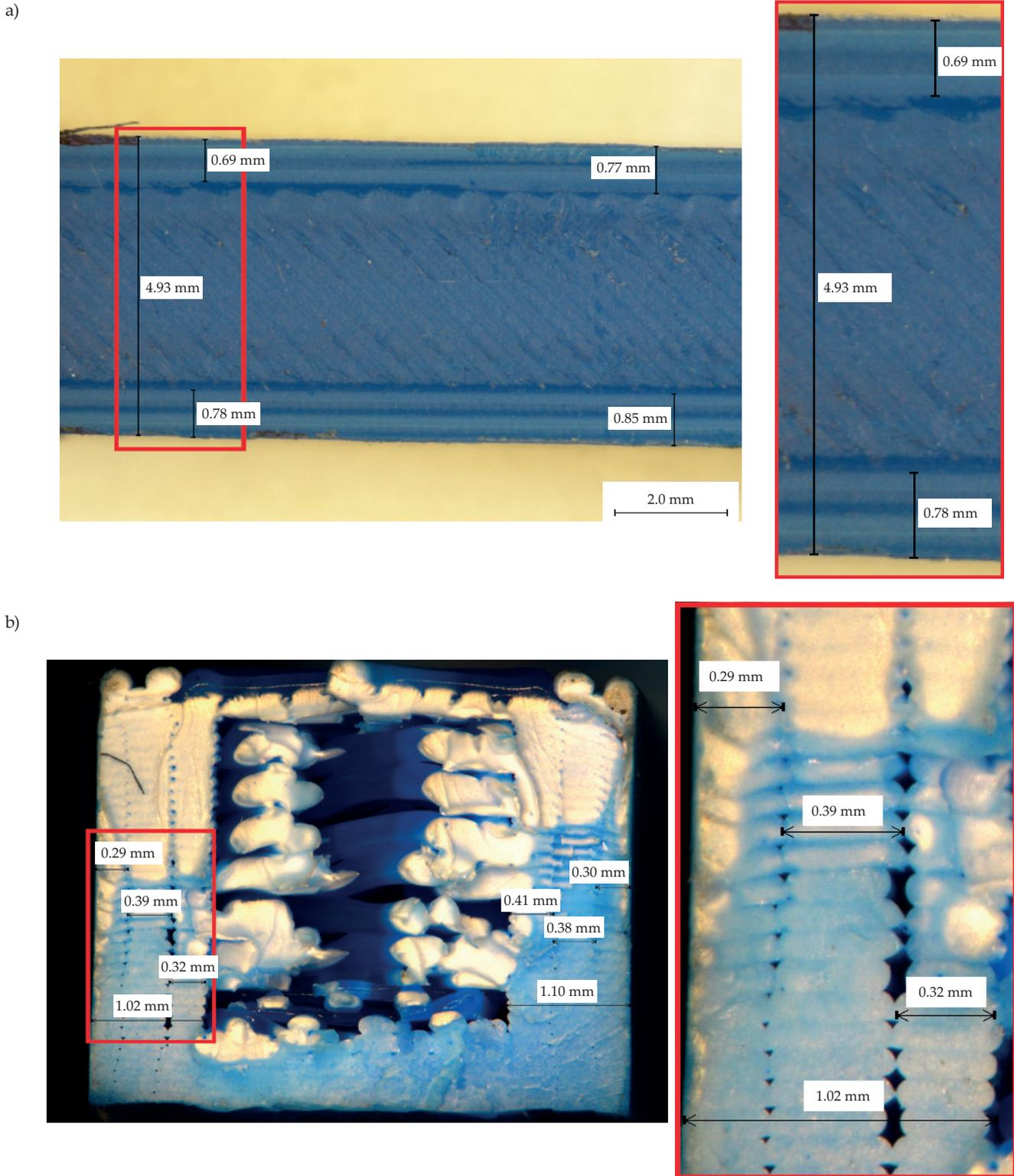
Fig. 3. Images of 3-shell sample: a) after machining, b) cross-section after the tensile test
