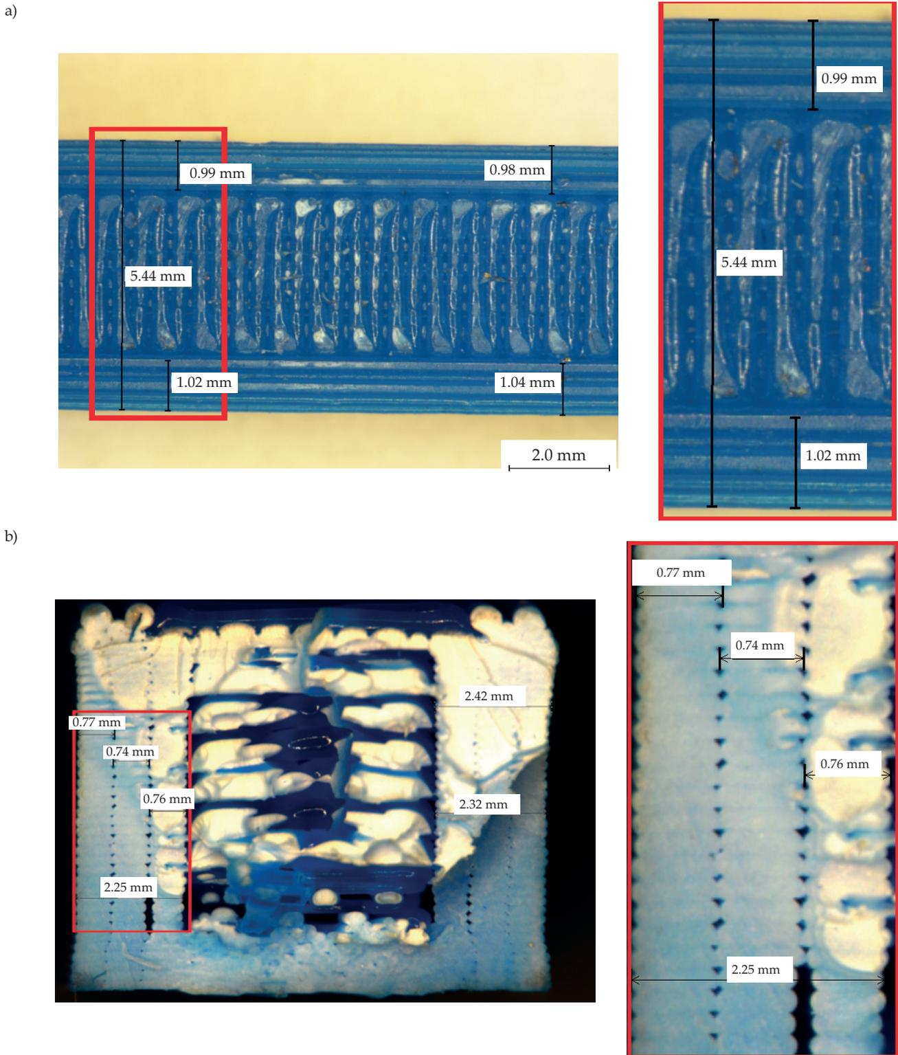
Fig. 2. Images of 3-shell sample: a) without machining, b) cross-section after the tensile test
