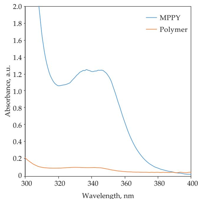
**Fig. 4.** UV-absorption of MPPY (0.85 mM) and PMMA in dichloromethane
