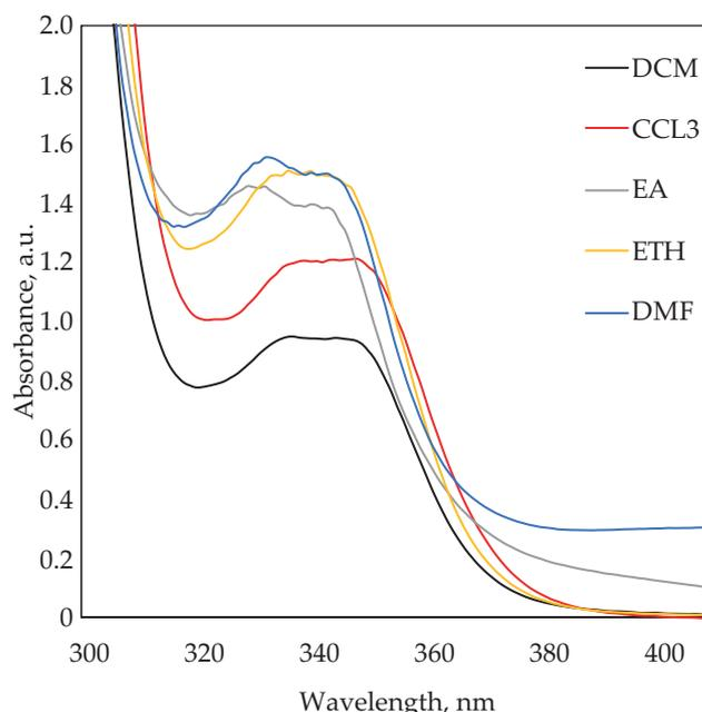
**Fig. 2. UV-absorption spectra of MPPY (0.85 mM) in various solvents**
