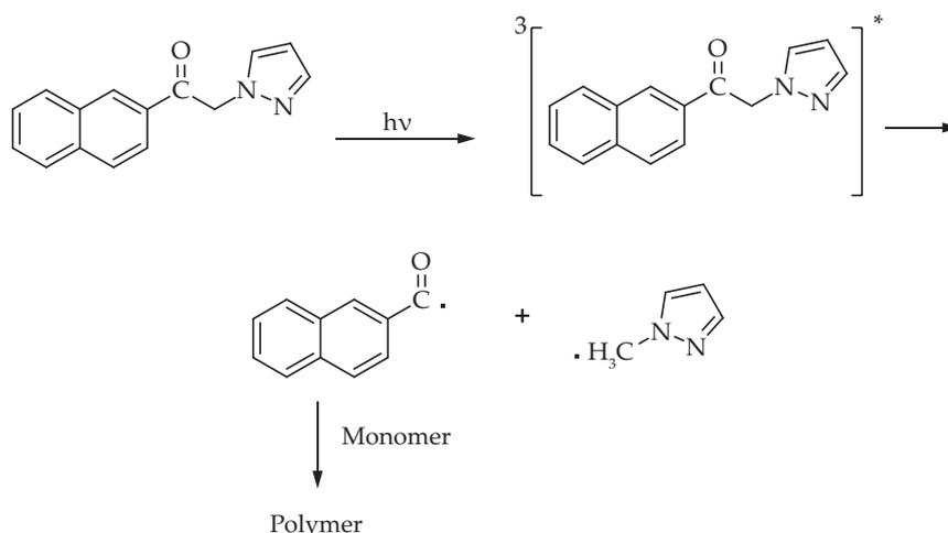
Fig. 5. Proposed MPPY photoinitiation mechanism
