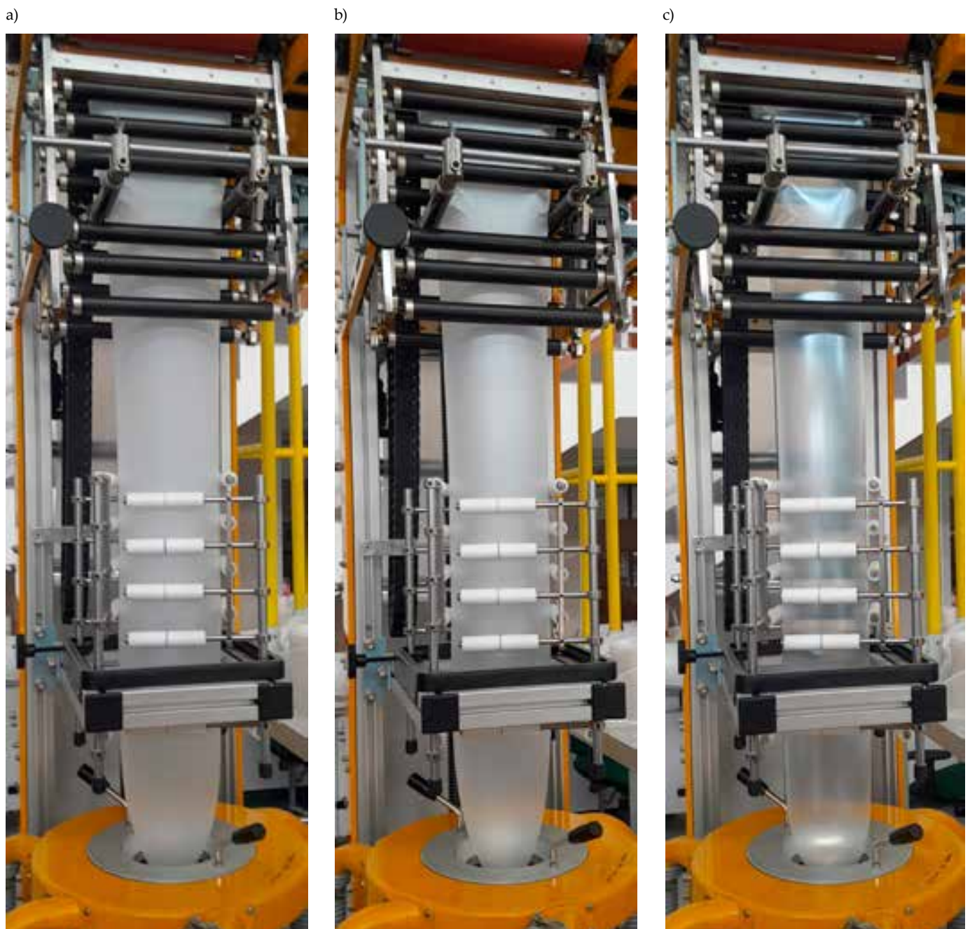
Fig. 4. Film blowing process of PLA/PBAT: a) 30/70, b) 50/50 c) 70/30
