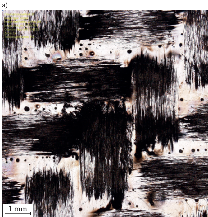
Fig. 7. Microscopic images of the damage center of EP_0.5%/CB/CF composite: a) one impulse, b) five impulses; 35× magnification
