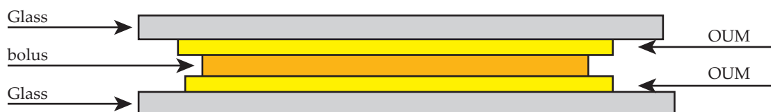
Fig. 6. Schematic diagram of the mold for preparing the PUM-bolus composite
