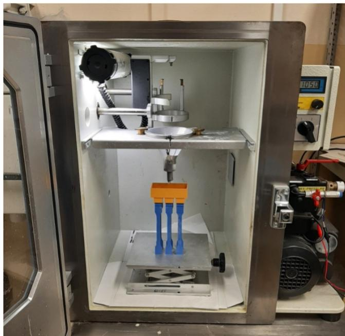
Fig. 7. Vacuum casting chamber
