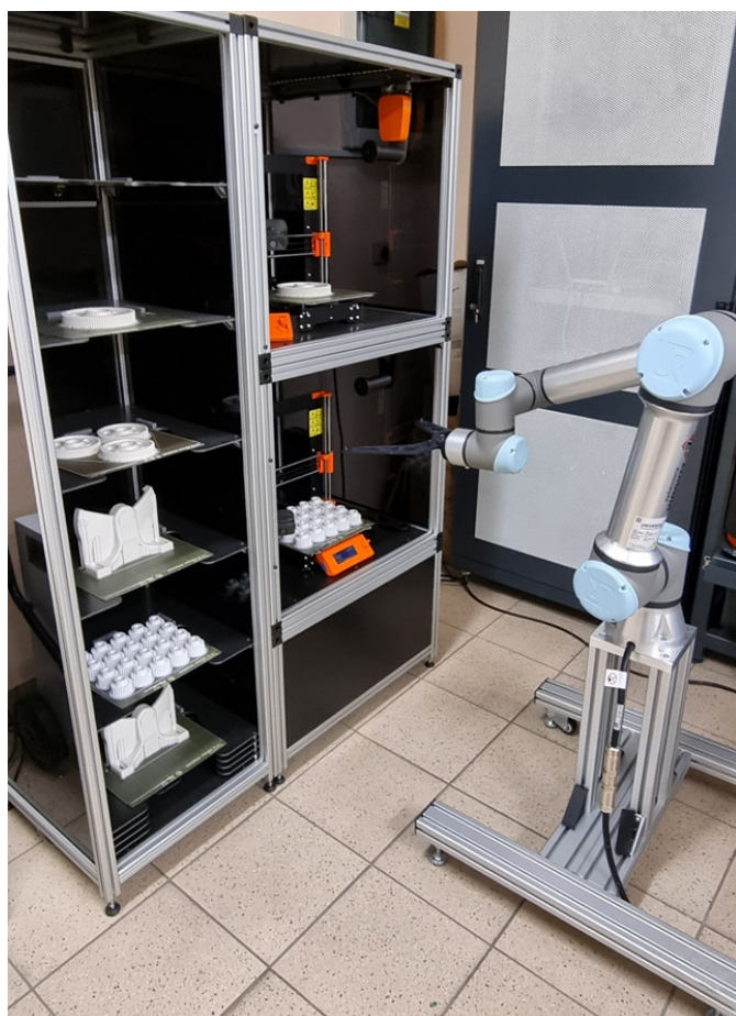
Fig. 2. Automated 3D printing station for layered extrusion of polymer materials
