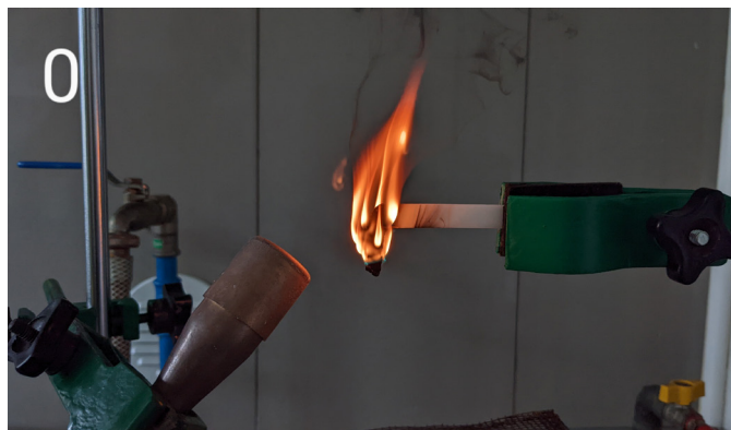
Fig. 2. Combustion test of reference sample
