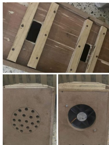
Fig. 3. View of the filter box
