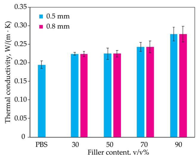
Fig. 6. Thermal conductivity of composites
