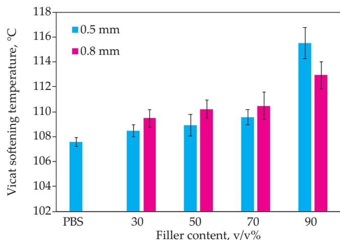
Fig. 7. Vicat softening temperature of composites
