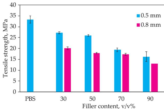
Fig. 2. Tensile strength of composites
