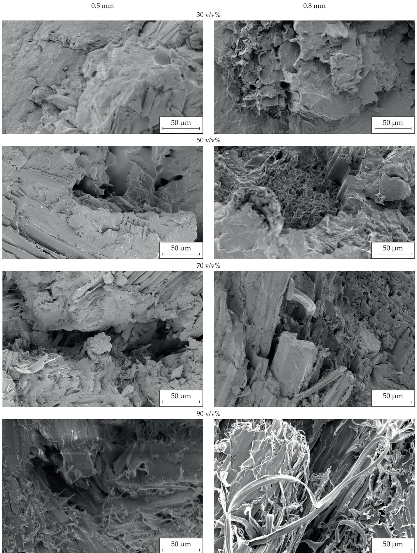
Fig. 4. SEM images of composites with different filler contents (30–90 v/v%) and dimensions (0.5 and 0.8 mm)
