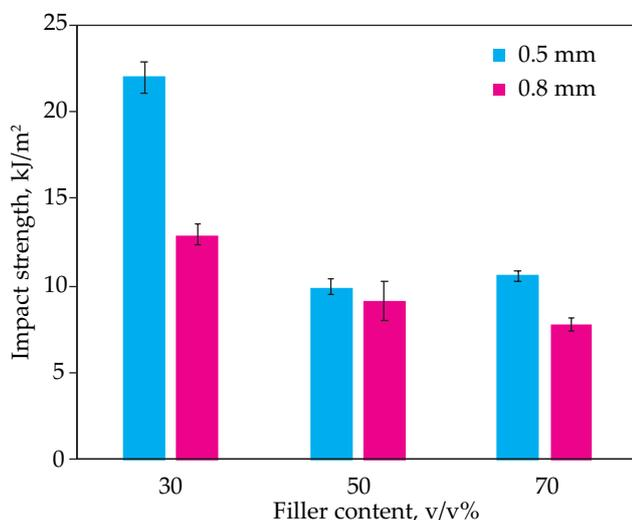
Fig. 5. Charpy unnotched impact strength of composites
