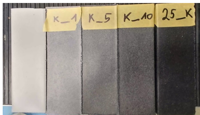
Fig. 2. Images of composites after rotational molding (from the left PP, then PP/xylite composites with different filler content)
