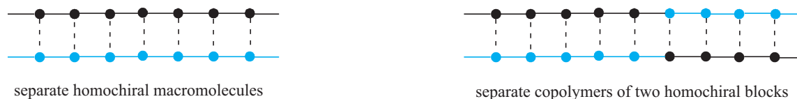
Scheme D. The pictograms of separate homochiral macromolecules and separate copolymers of two homochiral blocks, both forming stereocomplexes
