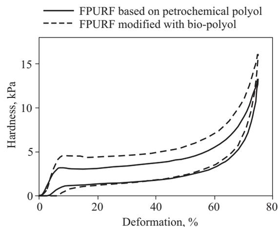
Fig. 2. Hysteresis loops of PUR foams (according to [70])
