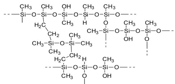
**Scheme G.** Chemical structure of polysiloxane microspheres produced from polysiloxanes with some hydromethyl groups
