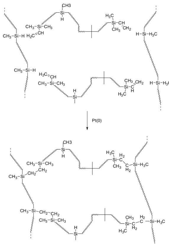
Scheme E. Cross-linking of polysiloxanes containing hydromethylsiloxane and vinyl groups
