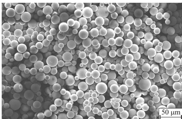
Fig. 5. SEM microphotograph of the cross-linked polysiloxane microspheres
